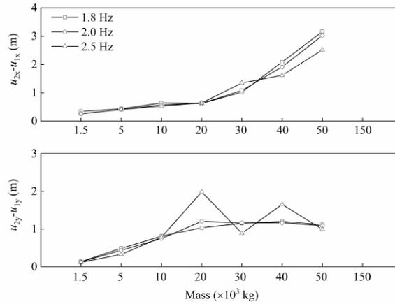
Fig. 8 – Relative horizontal displacements between vehicle and bridge when subject to earthquake record RSN1045
