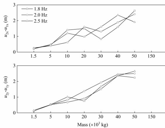
Fig. 7 – Relative horizontal displacements between vehicle and bridge when subject to earthquake record RSN126
