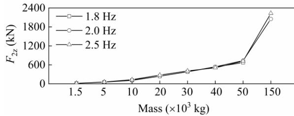
Fig. 6 – Vertical impact force between vehicle and bridge when subject to earthquake record RSN1531
