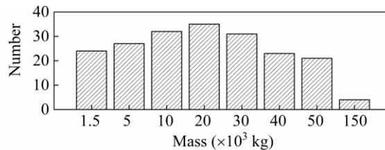
Fig. 3 – Histogram of impact cases distributed with vehicle mass
