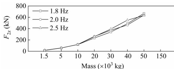
Fig. 4 – Vertical impact force between vehicle and bridge when subject to earthquake record RSN126
