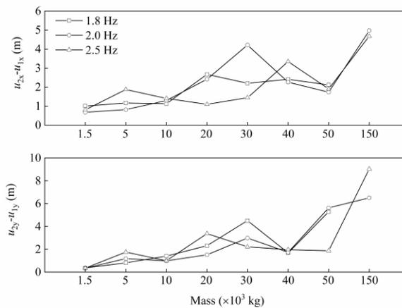
Fig. 9 – Relative horizontal displacements between vehicle and bridge when subject to earthquake record RSN1531
