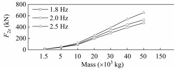
Fig. 5 – Vertical impact force between vehicle and bridge when subject to earthquake record RSN1045
