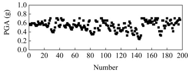
Fig. 2 – Distribution of peak ground acceleration when impact happening
