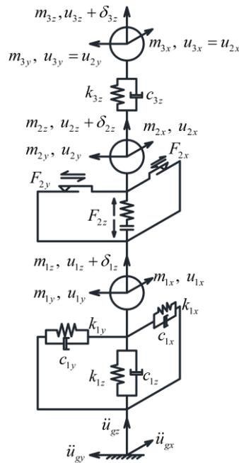
Fig. 1 – Simplified vehicle-bridge system
