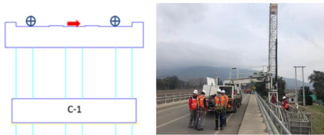
Fig. 7 – Sensor arrange during the third campaign
