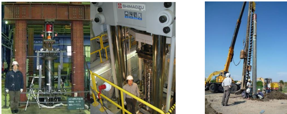
Fig. 10 – Development of bridge components according to the capacity design methodology: (a) steel tube column with high displacement ductility; and (b) ultra-high-strength prestress concrete pile with carbon fiber sheet [9, 12]
