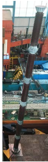
Fig. 7 – General overview of the post insulator
