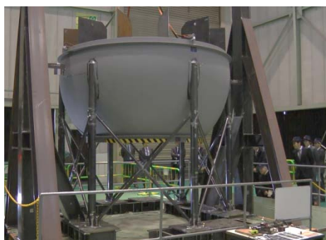
Photo 1 — 1G vibration test of spherical reservoir (steel tube brace) model [4]
