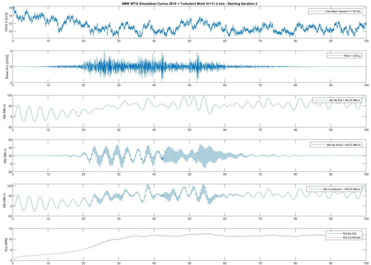
Fig. 4 – Idling Analysis Example (Wind Speed, Ground Acceleration, Base Moments for Wind, Earthquake and Combined Loads, Rotor Angular Speed).
