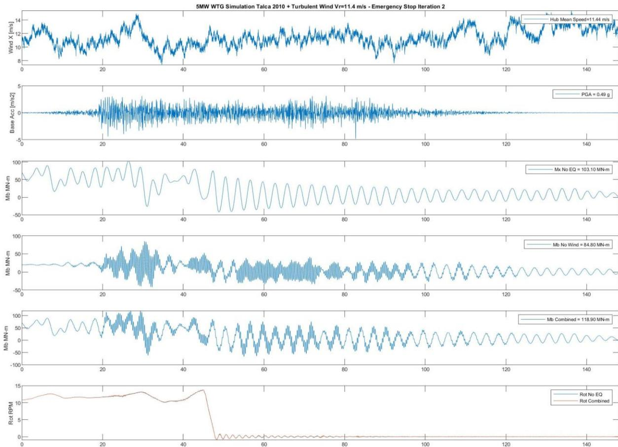
Fig. 3 – Emergency Stop Analysis Example (Wind Speed, Ground Acceleration, Base Moments for Wind, Earthquake and Combined Loads, Rotor Angular Speed).
