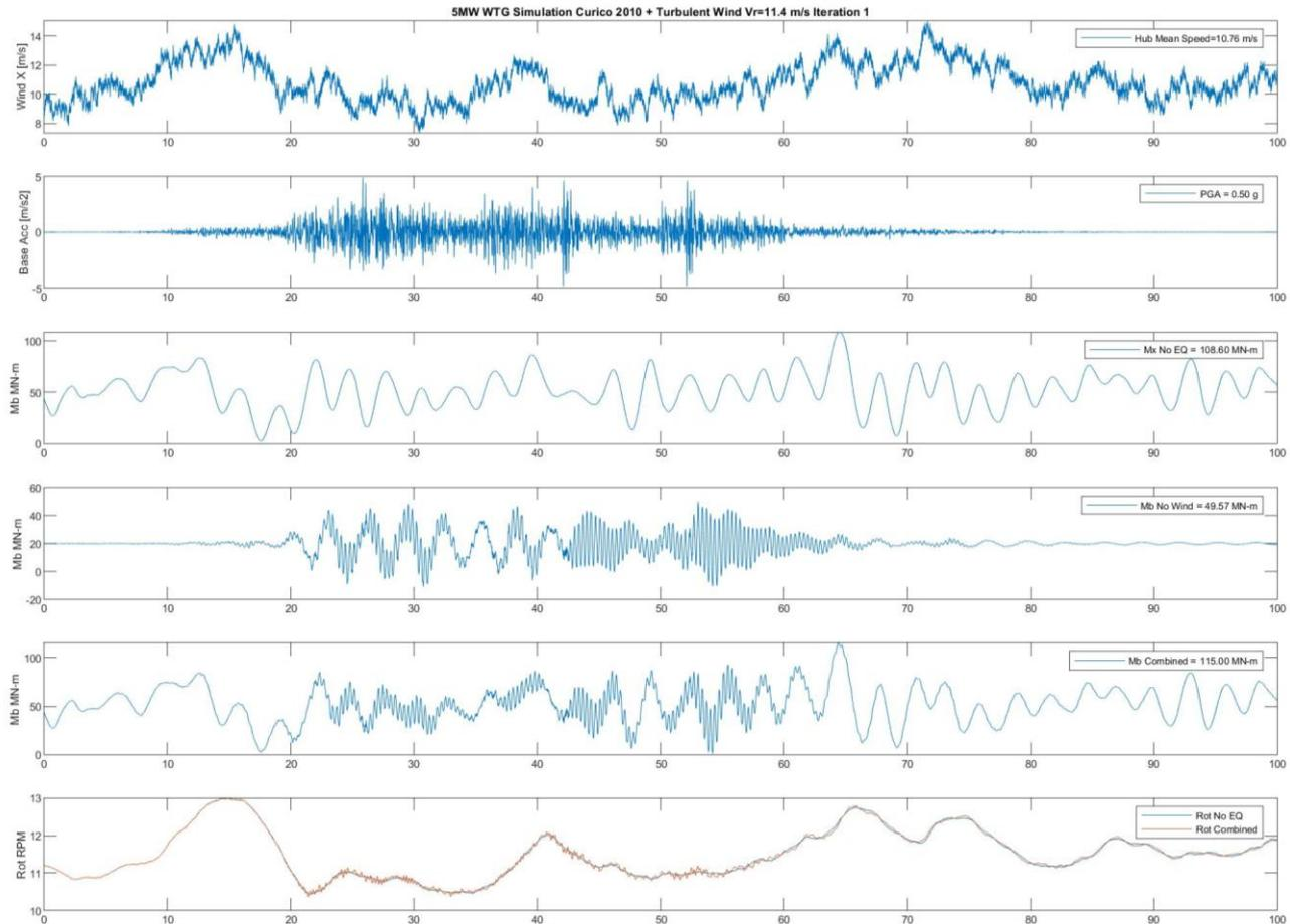
Fig. 2 – Normal Operation Analysis Example (Wind Speed, Ground Acceleration, Base Moments for Wind, Earthquake and Combined Loads, Rotor Angular Speed).
