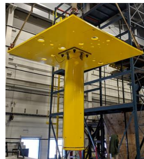
(b) central internal component: round HSS 12.75 × 0.25 steel pipe [11], radius of 0.162 m, height of 1.5 m, wall thickness of 6.35 mm
