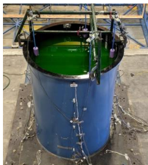
(a) base-supported steel tank filled with water: radius of 0.79 m, height of 2 m, wall thickness of 8 mm
