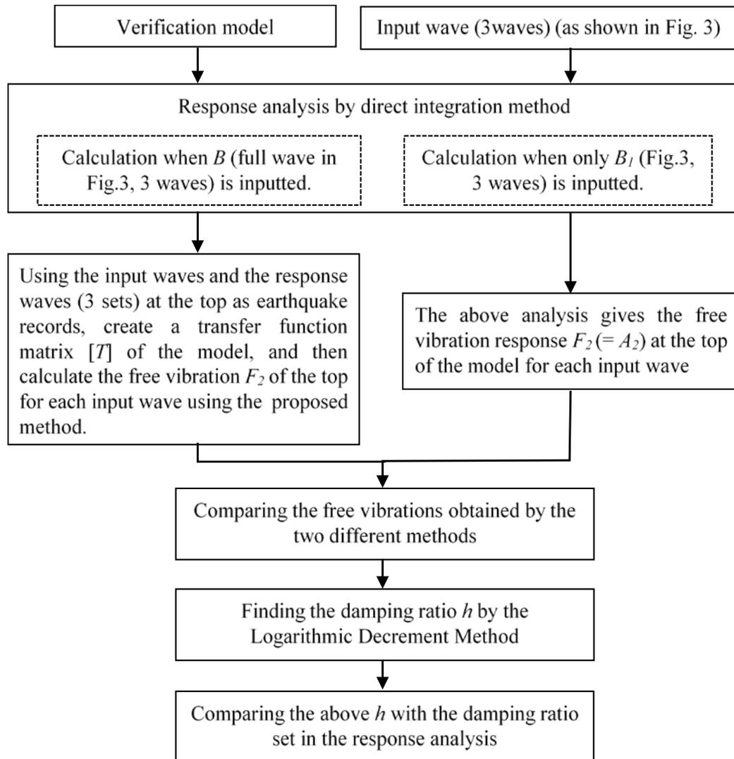
Fig. 6 - Flow of verification analysis
