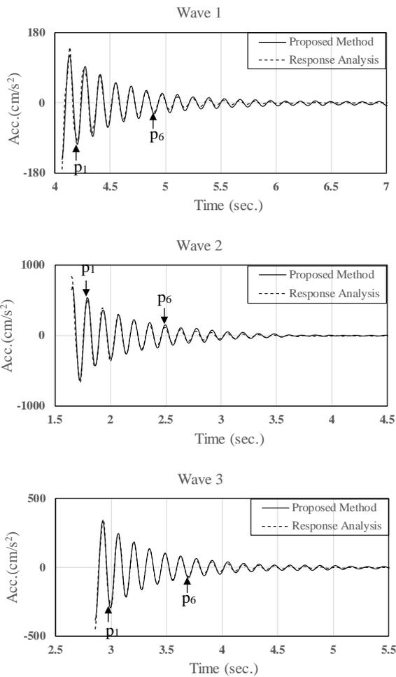
Fig. 11 - Comparison of the free vibration obtained by the proposed method and response analysis
