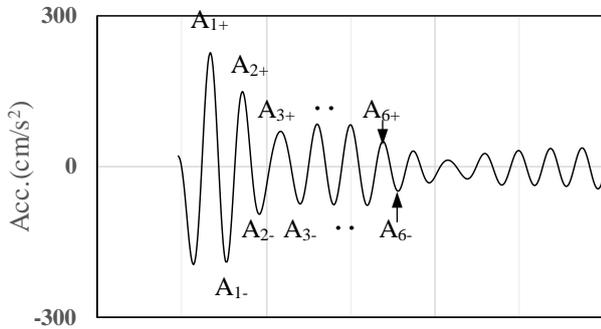
Fig. 14 – Example of the waveform obtained as free vibration of an existing dam
