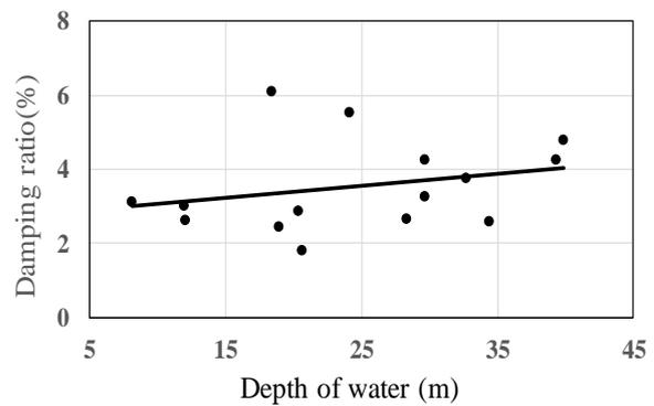
Fig. 17 - Relationship of water depth & damping ratio
