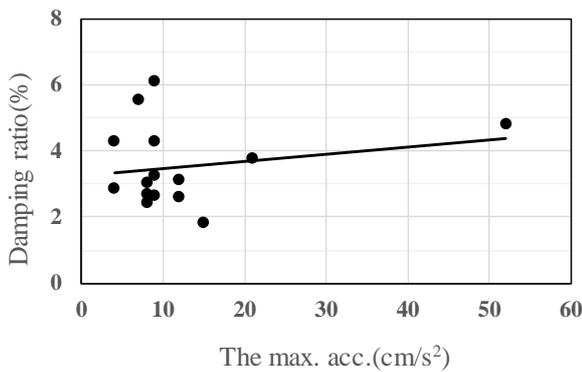
Fig. 16 - Relationship of peak acc. & damping ratio
