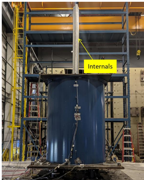
a. internals of Test 4C attached to the vessel head for hammer impact tests
