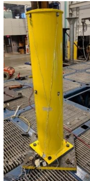
b. steel internal bolted to the earthquake simulator
