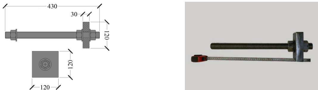
Fig. 1 – Investigated cast-in-place anchors: (a) Schematic drawing; (b) picture of a sample.
