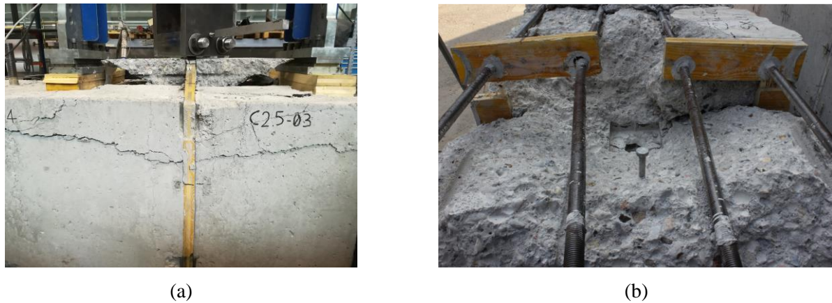
Fig. 8 – Concrete cone geometry: (a) failure surface parallel to bending span, (b) failure surface perpendicular to bending span.
