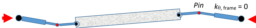
Figure 3. Out-of-Plane Frame Deformation of Idealised BRB with End Pins and Flexible Boundaries
