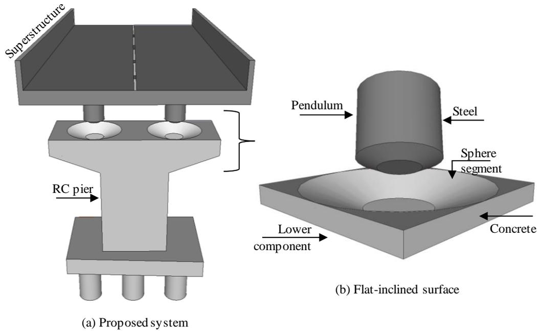
Fig. 1 – Proposed RC bridge pier with a spherical flat-inclined surface
