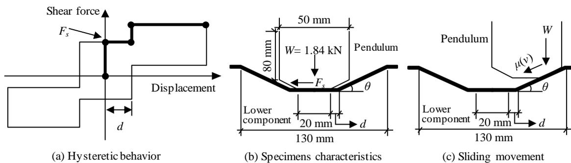
Fig. 2 – Hysteretic behavior and characteristics of specimen
