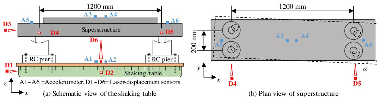
Fig. 3 – Characteristics of the bridge model
