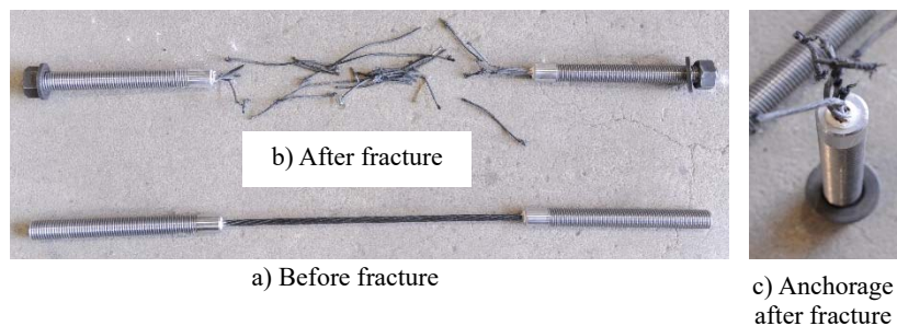
Fig. 4 - Images from CFCC coupon tests (a) before fracture (b) after fracture (c) anchorage after fracture
