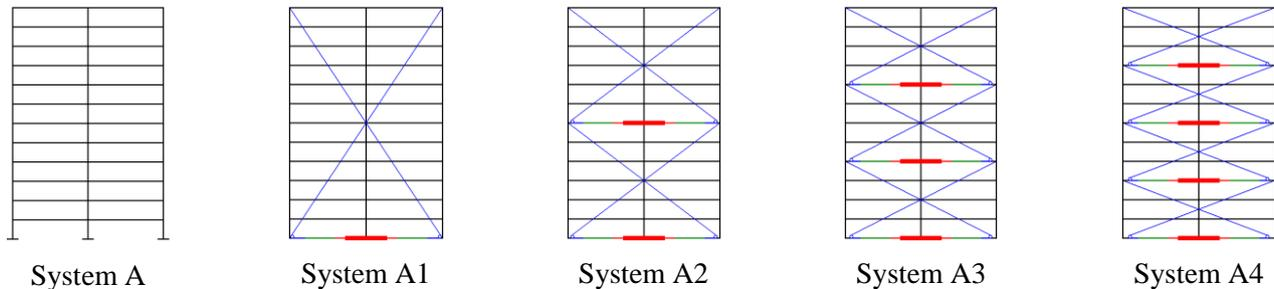
Fig. 4 Distribution of the resettable devices
