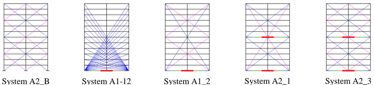
Fig. 6 Configuration of the tendon systems
