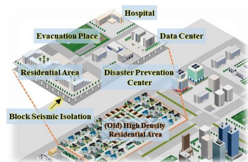
Fig. 1 – Seismic isolation block concept
