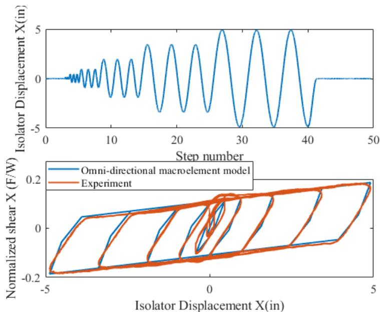
Fig. 6 – Controlled-displacement sine-wave orbits and experimental and numerical hysteresis loops
