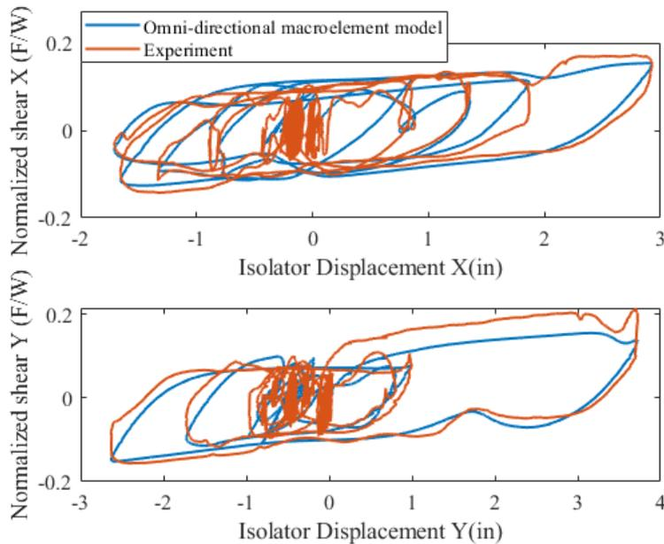
Fig. 10 – Experimental and numerical hysteretic curves for the Northridge earthquake Newhall record
