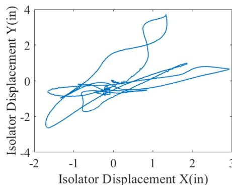
Fig. 9 – Uncontrolled-displacement orbits from the Northridge earthquake Newhall record
