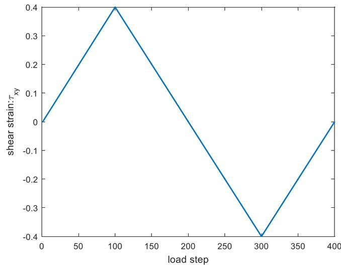
Fig. 2 – The displacement loading protocol
