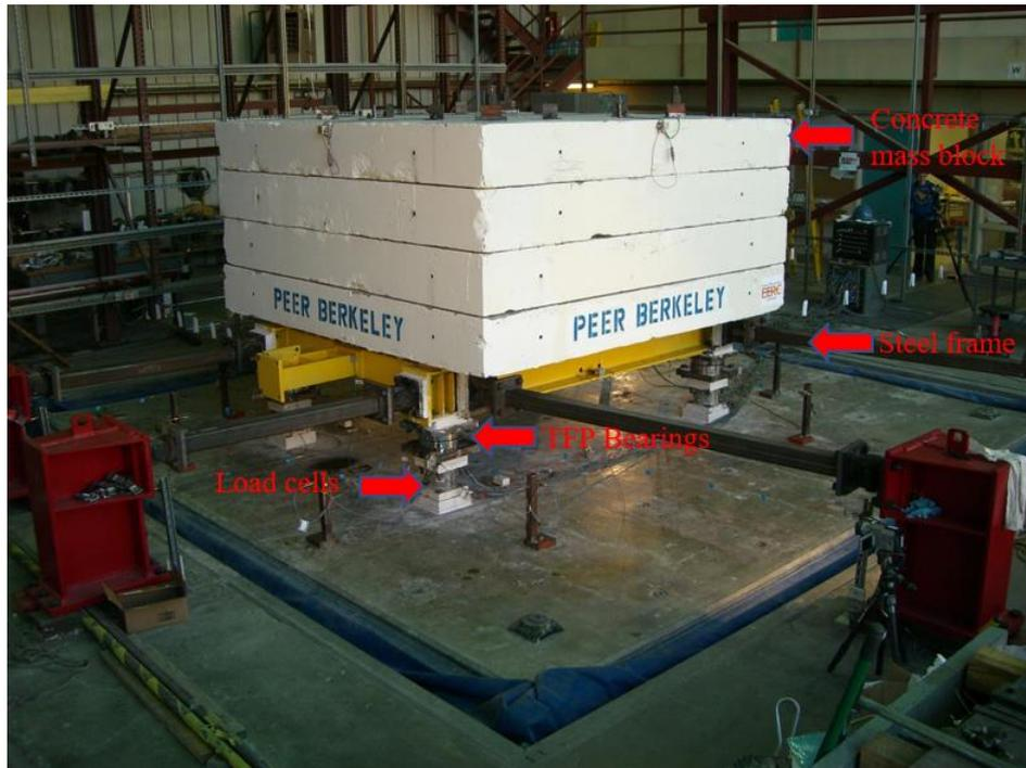
Fig. 4 – Rigid block set up at the UC Berkeley PEER Earthquake Simulator (adapted from [7])
