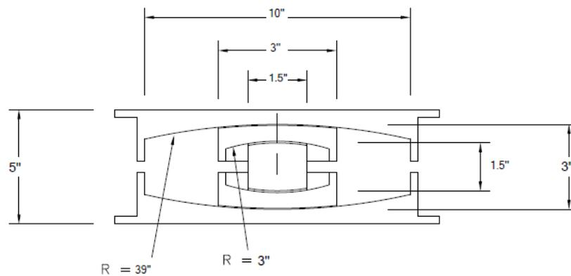
Fig. 5 – Section view of the TFP bearing
