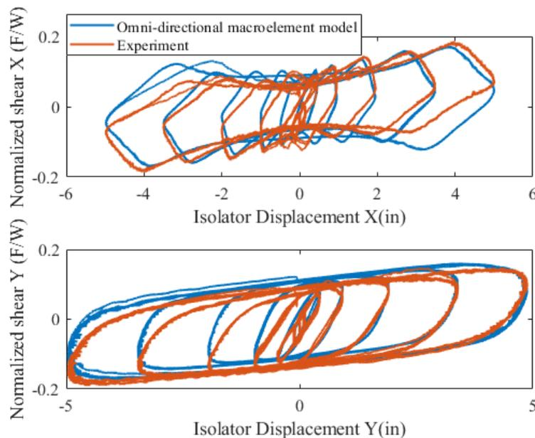
Fig. 8 – Experimental and numerical hystereses for the figure eights displacement orbit
