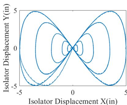
Fig. 7 – Controlled-displacement eight displacement orbit
