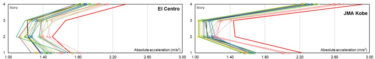
Fig. 8 – Maximum absolute acceleration for each floor in response to level 2 observed earthquakes.
