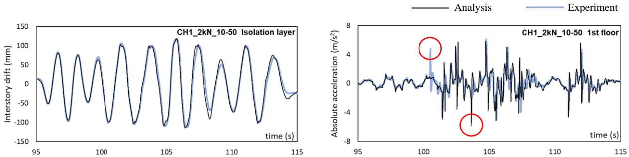
Fig. 13 – Enlarged graph of time history waveforms obtained by test results and numerical analysis results for absolute acceleration (CH1, (10, 50) initial clearance lengths, and 2 kN air cylinders).
