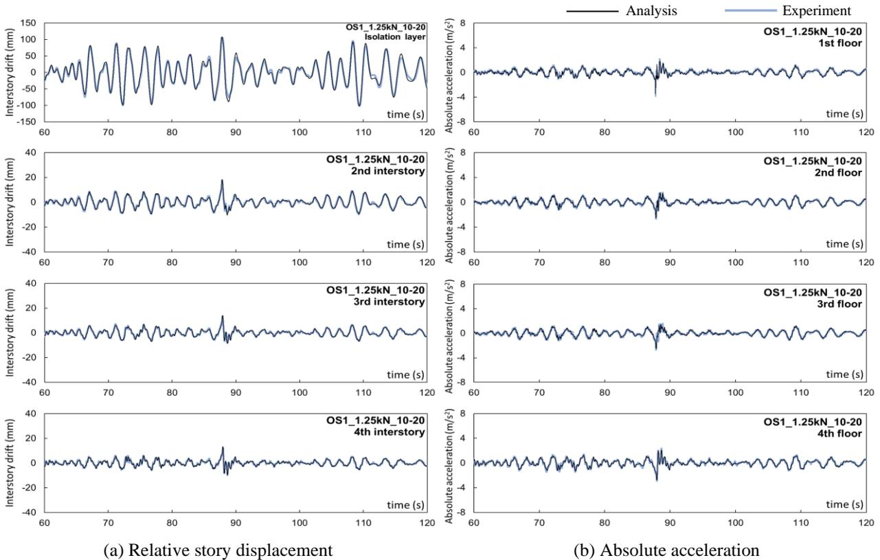
Fig. 9 – Time history waveforms of test results and numerical analysis results (OS1, (10, 20) initial clearance lengths, and 1.25 kN air cylinders).
