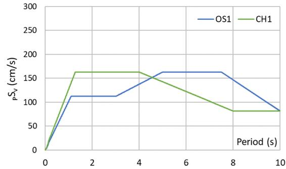
Fig. 4 – Velocity response spectrum of OS1 and CH1 ground motions on engineering bedrock for 5% damping factor.
