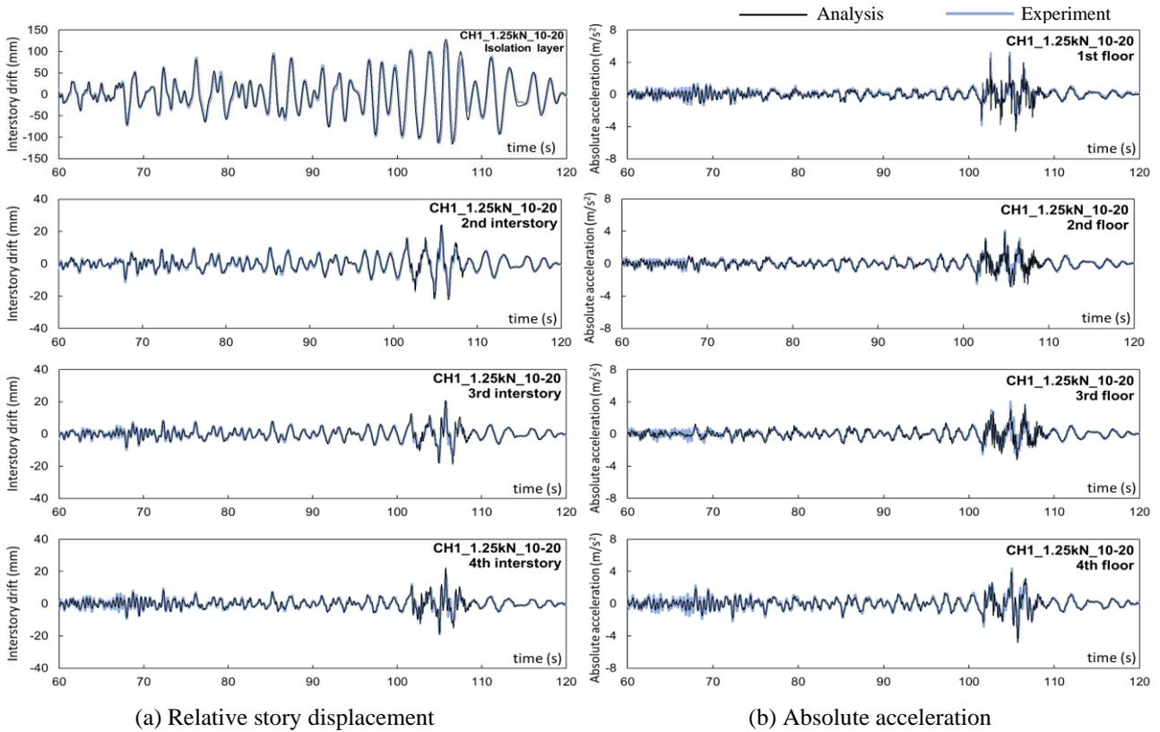
Fig. 11 – Time history waveforms of test results and numerical analysis results (CH1, (10, 20) initial clearance lengths, and 1.25 kN air cylinders).
