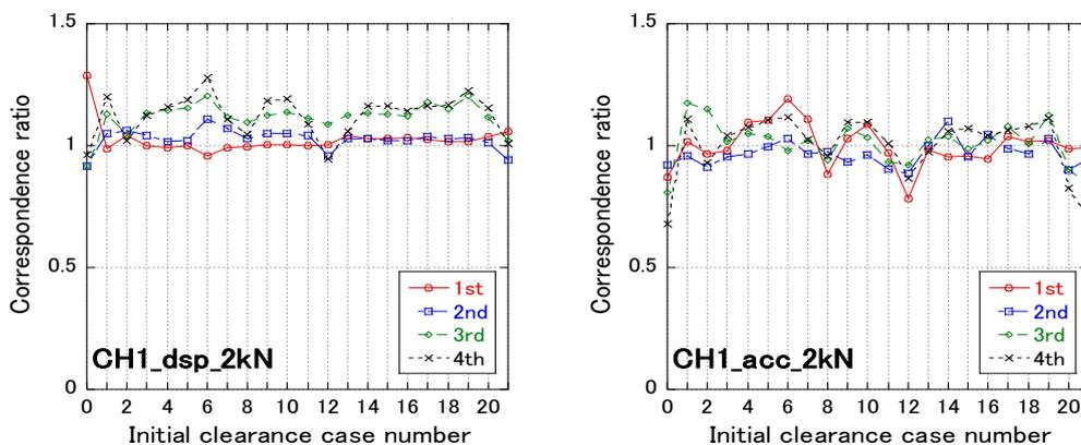
Fig. 17 – Ratios of analytical maximum response divided by test results for relative story displacement (left panel) and absolute acceleration (right panel) responses, respectively, to CH1, for each floor and all initial clearance combination cases, with 2 kN air cylinder.
