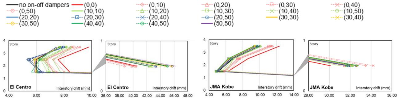
Fig. 7 – Maximum relative story displacement for each floor in response to level 2 observed earthquakes.
