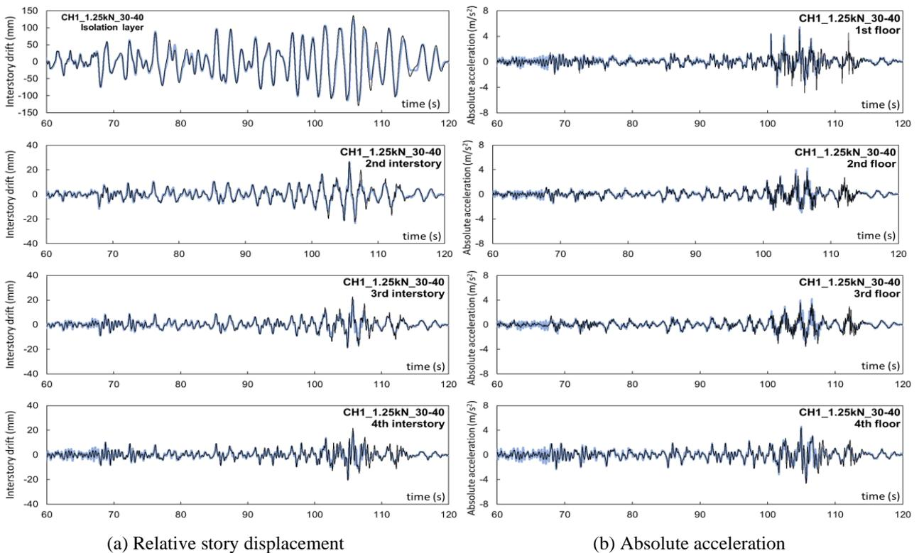
Fig. 12 – Time history waveforms of test results and numerical analysis results (CH1, (30, 40) initial clearance lengths, and 1.25 kN air cylinders).
