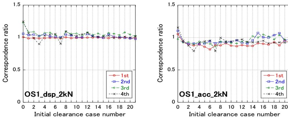
Fig. 15 – Ratios of analytical maximum response divided by test results for relative story displacement (left panel) and absolute acceleration (right panel) responses, respectively, to OS1, for each floor and all initial clearance combination cases, with 2 kN air cylinder.
