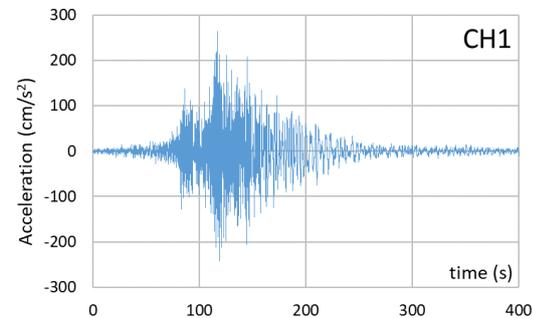
Fig. 3(b) – Time history waveforms of input accelerations from two estimated long-period and long-duration earthquake ground motions (OS1 and CH1 on engineering bedrock).
