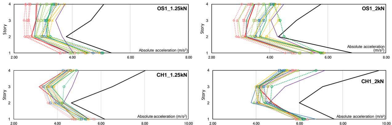
Fig. 6 – Maximum absolute acceleration for each floor in response to OS1 and CH1 ground motions, and 1.25 kN and 2 kN of ideal resultant output force.
