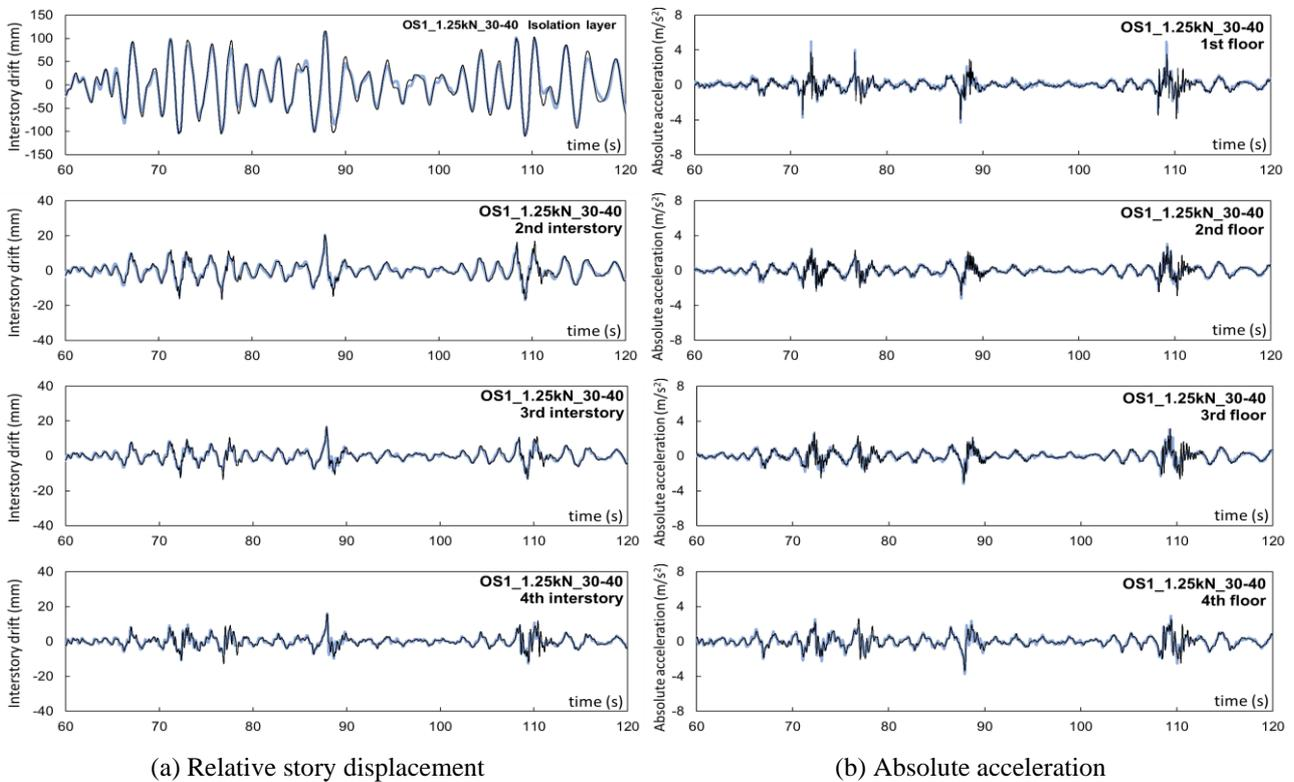
Fig. 10 – Time history waveforms of test results and numerical analysis results (OS1, (30, 40) initial clearance lengths, and 1.25 kN air cylinders).
