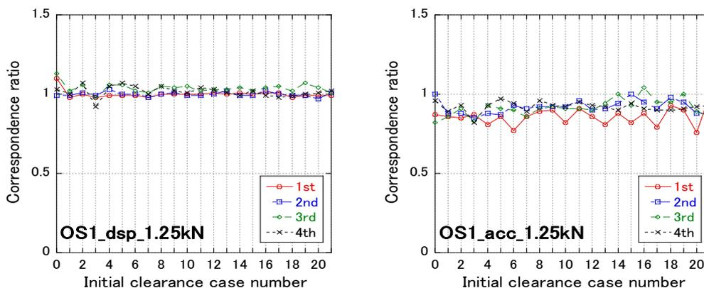
Fig. 14 – Ratios of analytical maximum response divided by test results for relative story displacement (left panel) and absolute acceleration (right panel) responses, respectively, to OS1, for each floor and all initial clearance combination cases, with 1.25 kN air cylinder.
