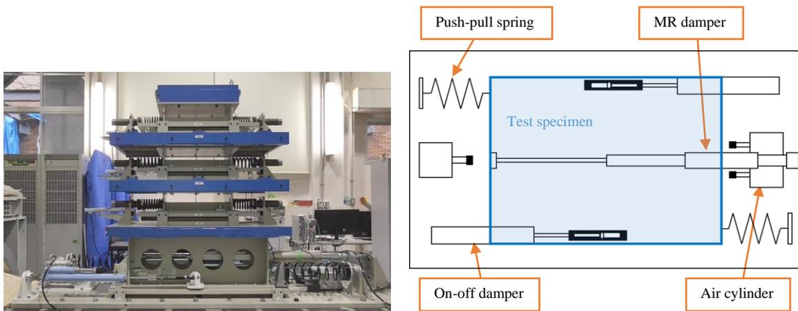
Fig. 2 – Experimental setup showing the four-story test structure (left) and setup plan (right).
