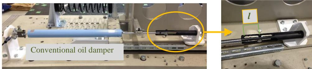
Fig. 1 – On-off damper used in shaking table tests. Note the elongated hole in the damper joint, with the shown initial clearance length ( $l$ ).
