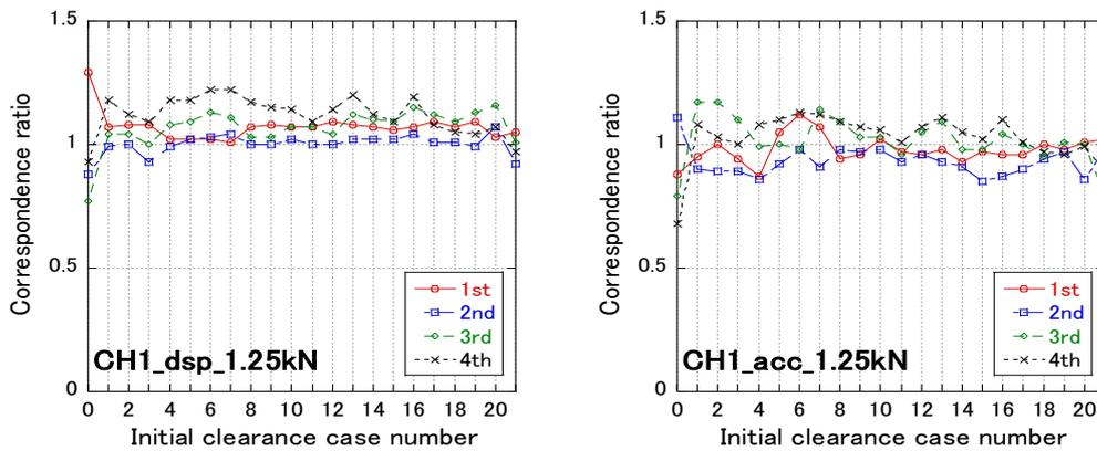
Fig. 16 – Ratios of analytical maximum response divided by test results for relative story displacement (left panel) and absolute acceleration (right panel) responses, respectively, to CH1, for each floor and all initial clearance combination cases, with 1.25 kN air cylinder.
