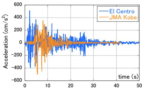
Fig. 3(a) – Time history waveforms of input accelerations from two observed earthquakes (1940 El Centro and 1995 JMA Kobe).
