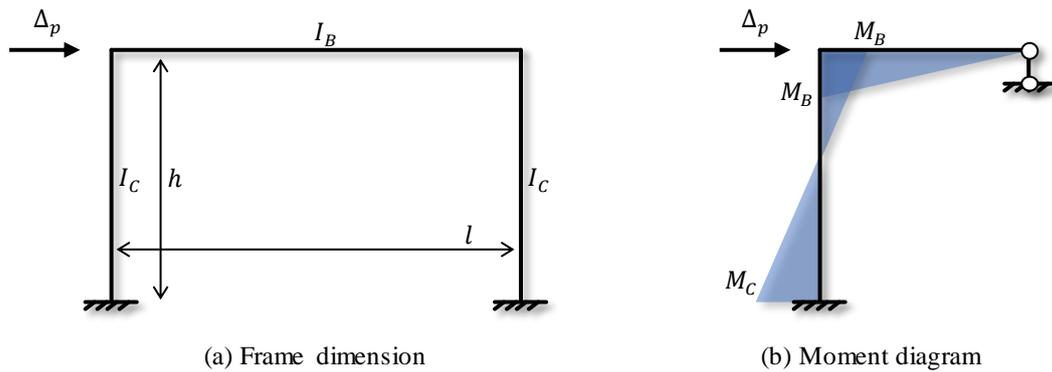
Fig. 3 –Force analysis of NCF under horizontal force
