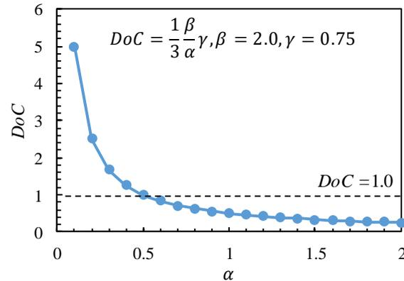
Fig. 5 –The influence of linear stiffness ratio of beam and column on  $DoC$
