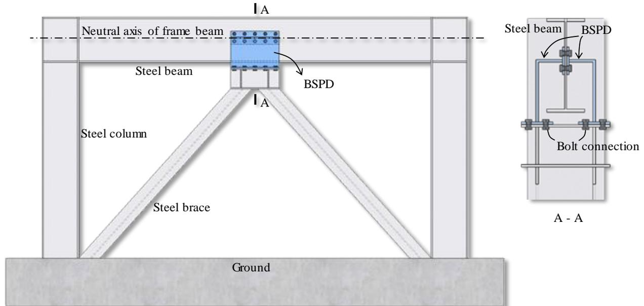
Fig. 9 – The configuration of BSPD in EBCF
