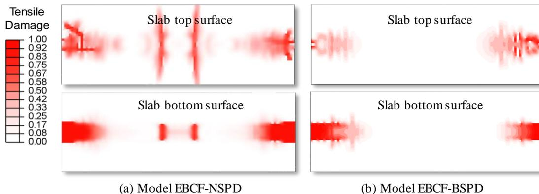
Fig. 17 Concrete slab damage distribution
