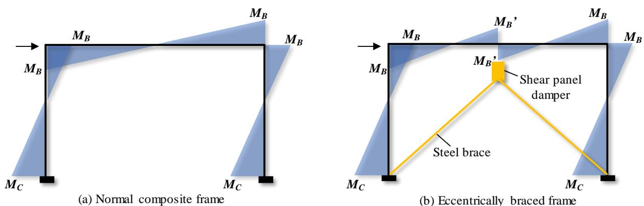
Fig. 2 – Moment diagram of different composite frame
