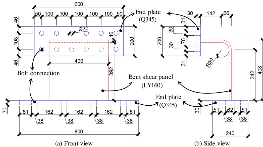
Fig. 13 – Dimension of test specimen
