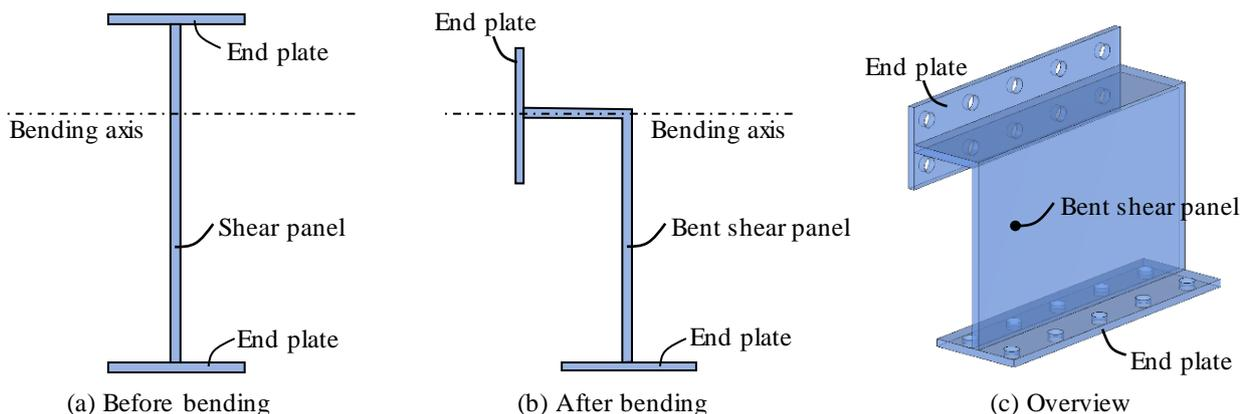
Fig. 8 – Bent shear panel damper (BSPD)
