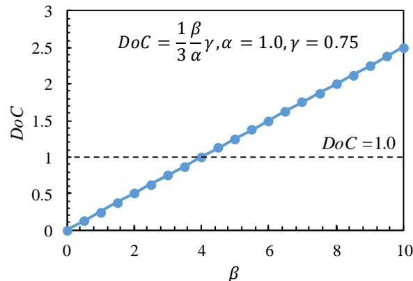
Fig. 6 –The influence of horizontal stiffness ratio of the bracing member and the frame on  $DoC$
