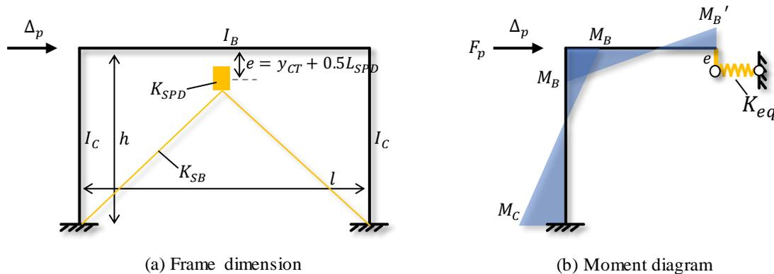
Fig. 4 – Force analysis of EBCF under horizontal force
