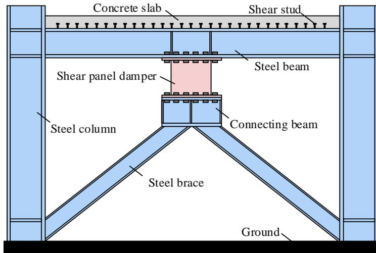
Fig. 1 – Typical configuration of eccentrically braced composite frame (EBCF)
