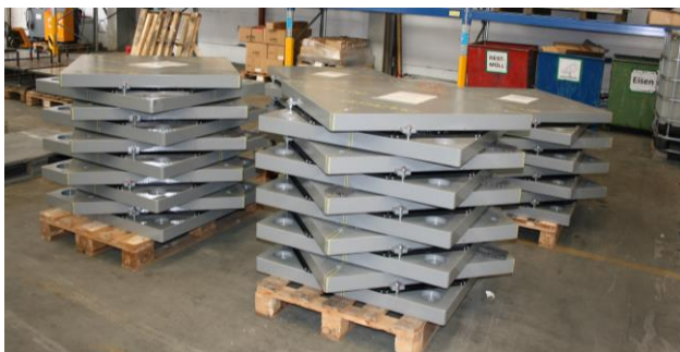
Fig. 11 – SIP D isolators ready for dispatch (left); positioning of isolator on plinth in the cellar level (right)
