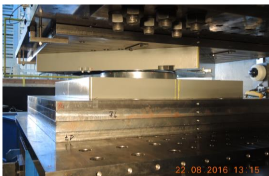
Fig. 9 – Prototype testing at EUCENTRE in Pavia (left); Integrity check of isolator after testing (right)
