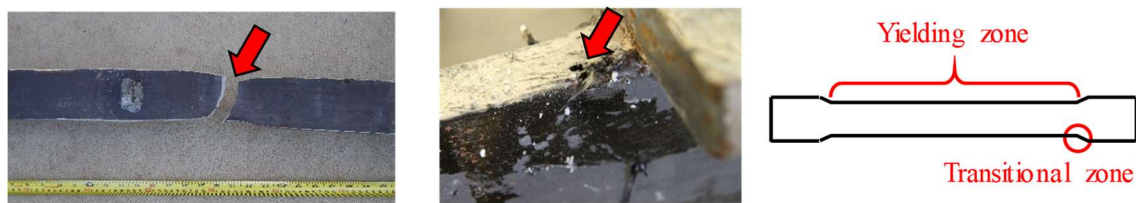
(a) Failure in the yielding zone (b) Failure in the transitional zone
