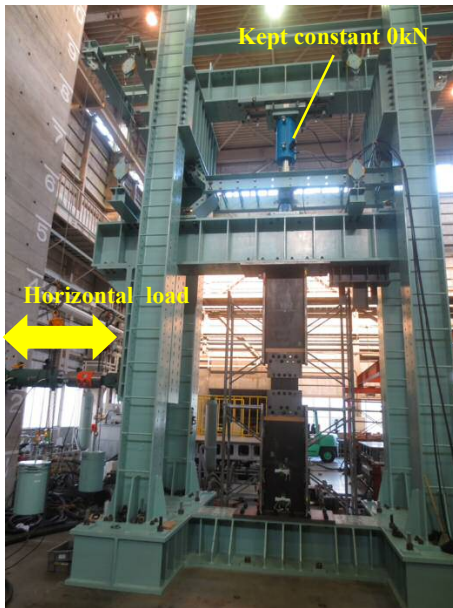
Photo 4 – Steel structure stud loading device
