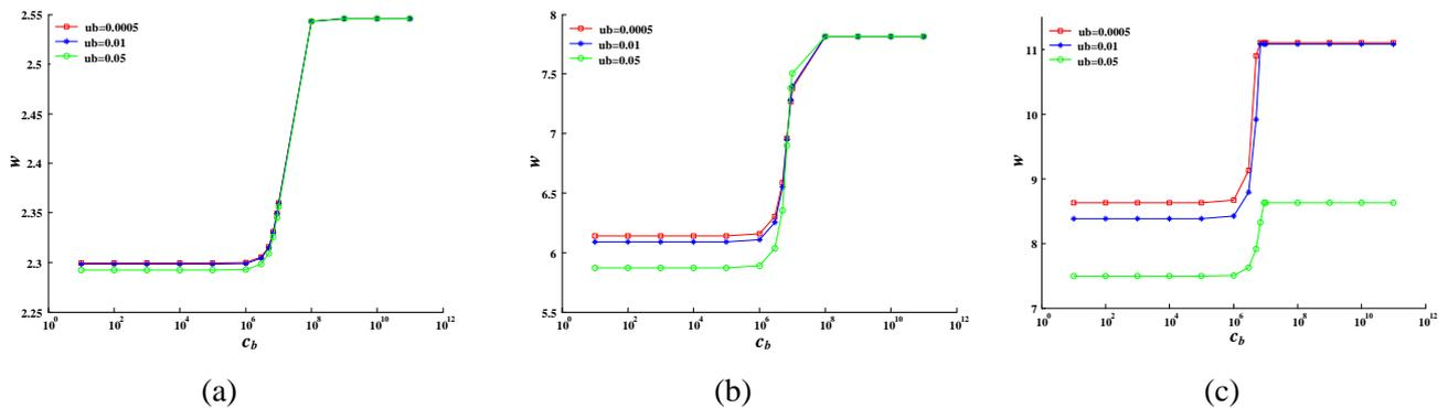
Fig. 4 –The relationship between the natural frequency of the system and the damping coefficient under different  $u_b$ : (a) first-order frequency, (b) second-order frequency, (c) third-order frequency.
