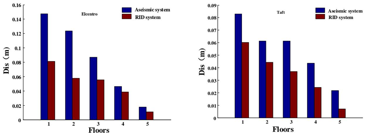
Fig. 6 – Comparison of the interlayer displacement of megastructure
