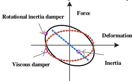
Fig. 2 – The relationship between force and deformation
