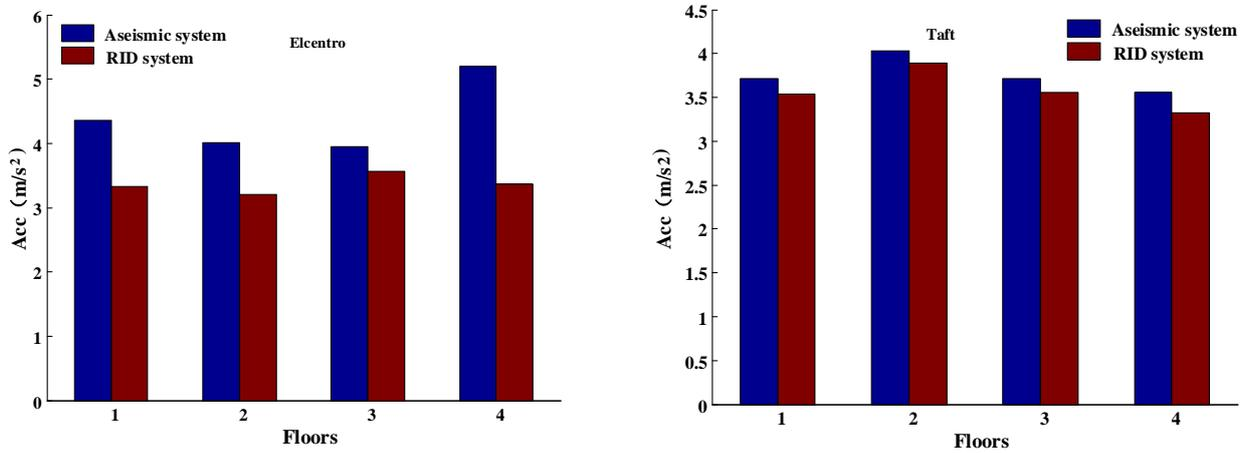
Fig. 8 – Comparison of the acceleration of substructure
