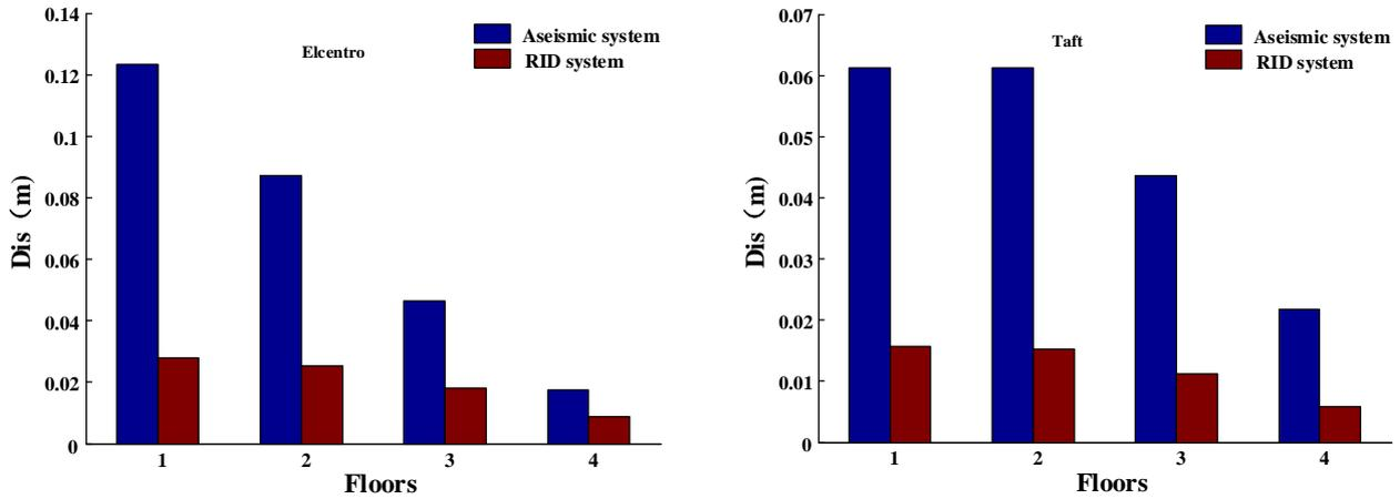
Fig. 7 – Comparison of the interlayer displacement of substructure
