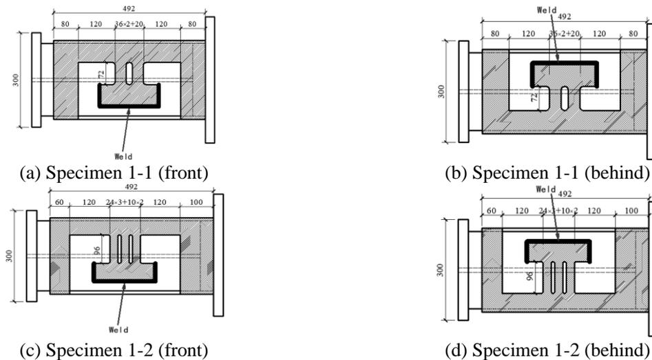
Fig. 7 Layout of tube damper specimens [20]
