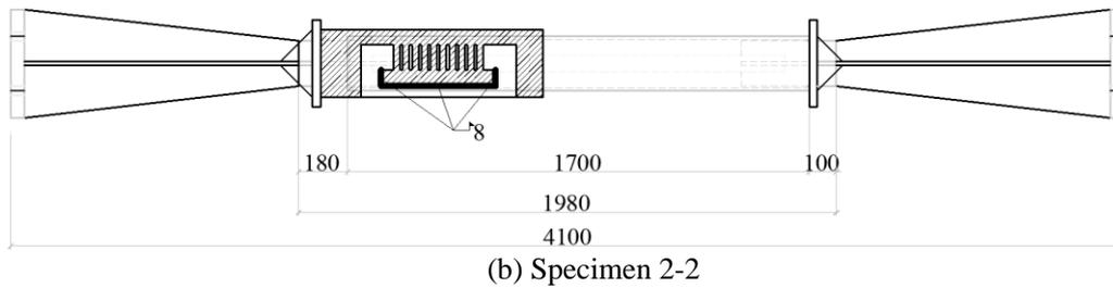
Fig. 11 Layout of two TYBRB specimens [19]
