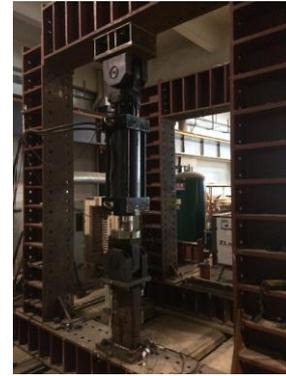
Fig. 9 Setup of steel tube damper specimens [20]
