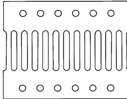
Fig. 3 Steel strip damper for Sapporo Art Center [6]
