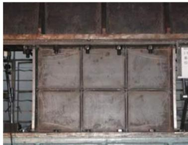
Fig. 4 Conventional shearing steel damper
