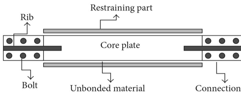
Fig. 5 Buckling restrained brace [18]
