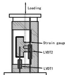
Fig. 8 Layout of measurements of steel tube damper specimens [20]
