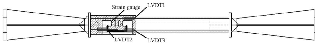
Fig. 12 Layout of measurements of TYBRB specimens [19]
