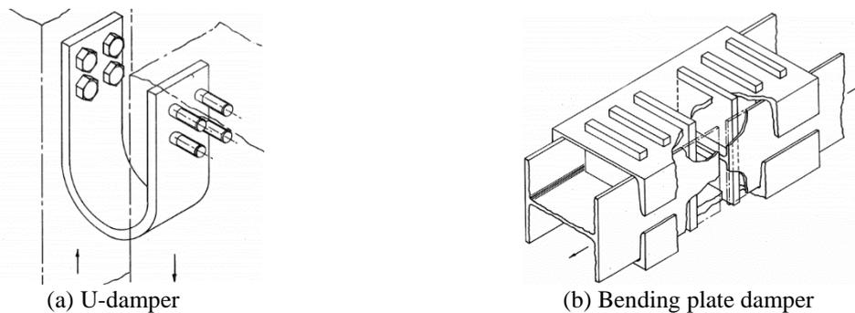
Fig. 1 Steel bending damper [2]
