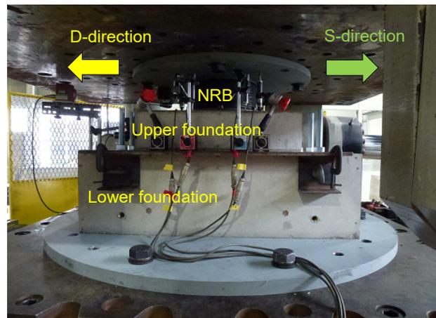
Fig.12 – NRB and RC specimen
