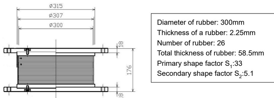
Fig.1 – Natural Rubber Bearing (unit: mm)
