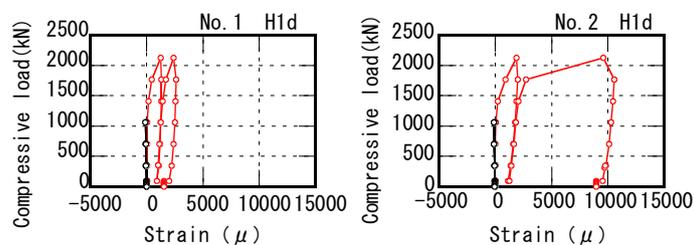
Fig.14 – Strain gauge H1d of shear reinforcement
