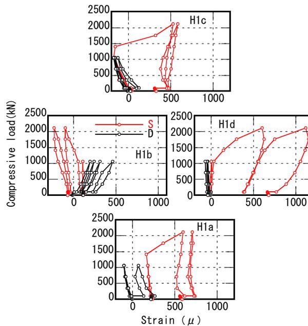
Fig.13 – Strain gauge H1a - H1d of shear reinforcement (RC specimen: No.3,  $F_c=30\text{MPa}$ )
