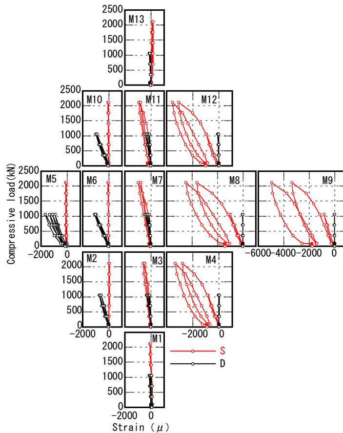
Fig.15 – Mold strain gauge M1 - M13 (RC specimen: No.3,  $F_c=30\text{MPa}$ )
