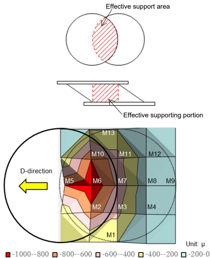
Fig.17 – Strain distribution of upper foundation
