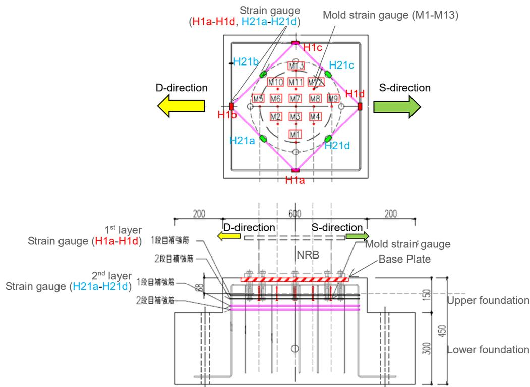
Fig.2 – Reinforced concrete foundation specimen No.2 (unit: mm)
