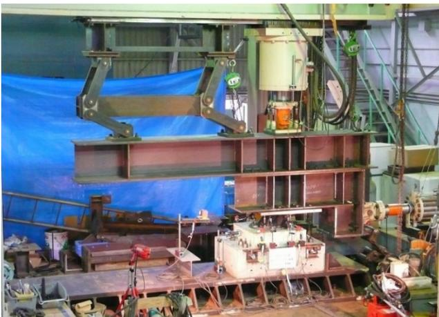
Fig.3 – Compressive shearing test machine 1
