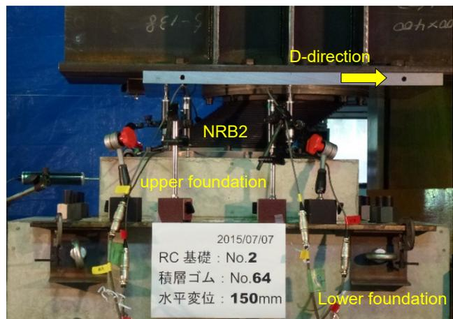
Fig.4 – RC specimen No.2 (NRB deformed 150mm)
