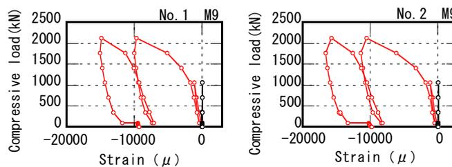
Fig.16 – Mold strain gauge M9 (RC specimen: No.1 and No.2,  $F_c=13.5\text{MPa}$ )
