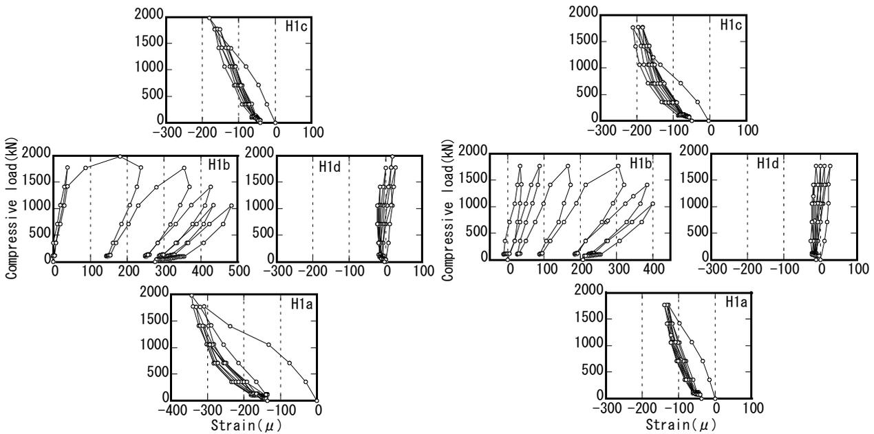
Fig.7–Strain gauge H1a - H1d of shear reinforcement (RC specimen: No.2,  $F_c=13.5\text{MPa}$ )
