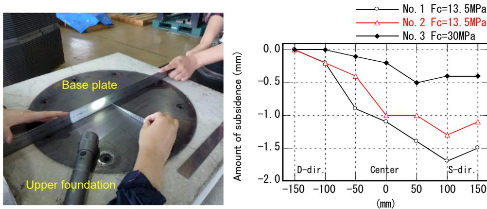
Fig.18 – Amount of subsidence of base plate
