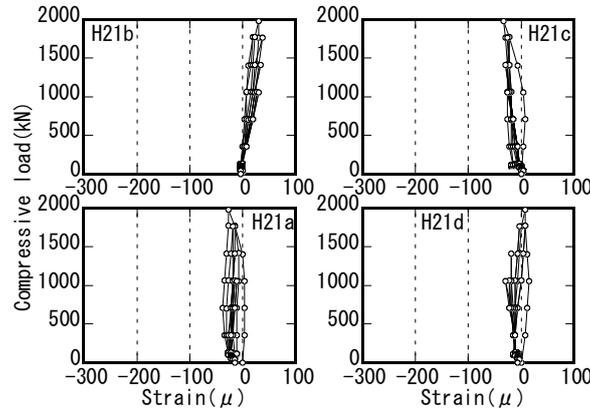
Fig.6 – Strain of shear reinforcement (Strain gauge: H21a - H21d, RC specimen: No.2)
