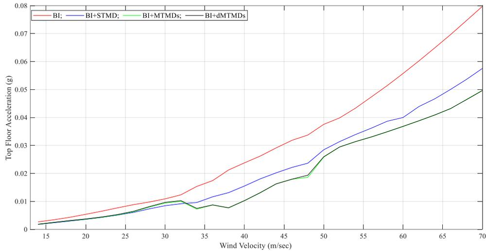
Fig. 3 – Variation of acceleration response with increasing wind velocity.
