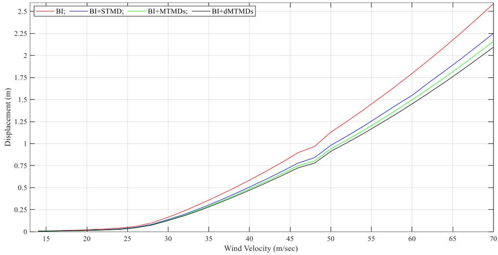
Fig. 2 – Variation of displacement response reduction with increasing wind velocity.
