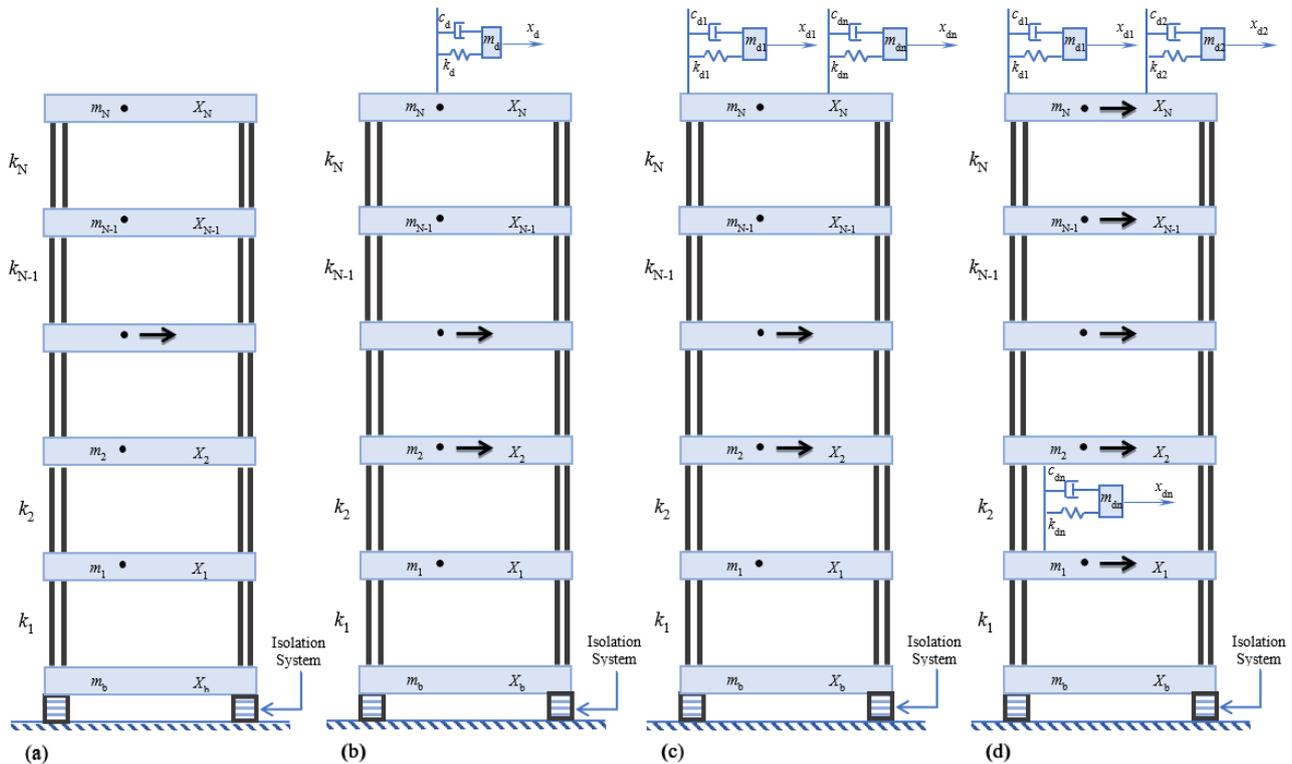
Fig. 1 – Mathematical model of a  $N$ -story building with (a) BI, (b) BI + STMD at top floor, (c) BI + MTMDs at top floor, and (d) BI+d-MTMDs.
