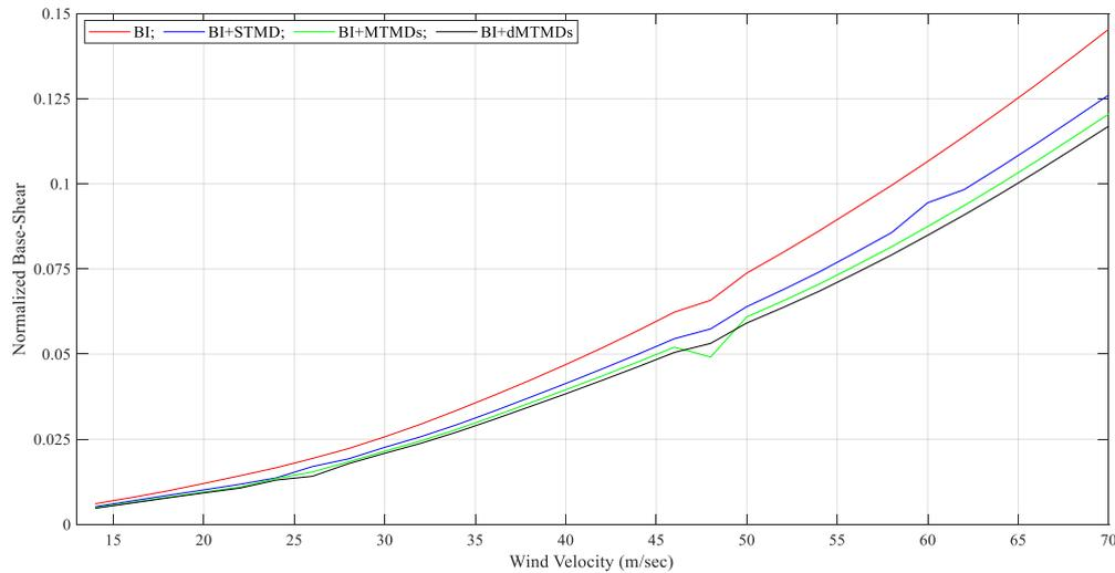
Fig. 4 – Variation of base-shear response with increasing wind velocity.
