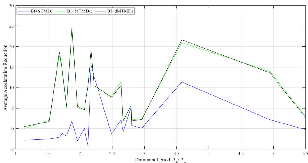
Fig. 6 – Variation of average reduction in peak roof acceleration for earthquakes with different dominant periods
