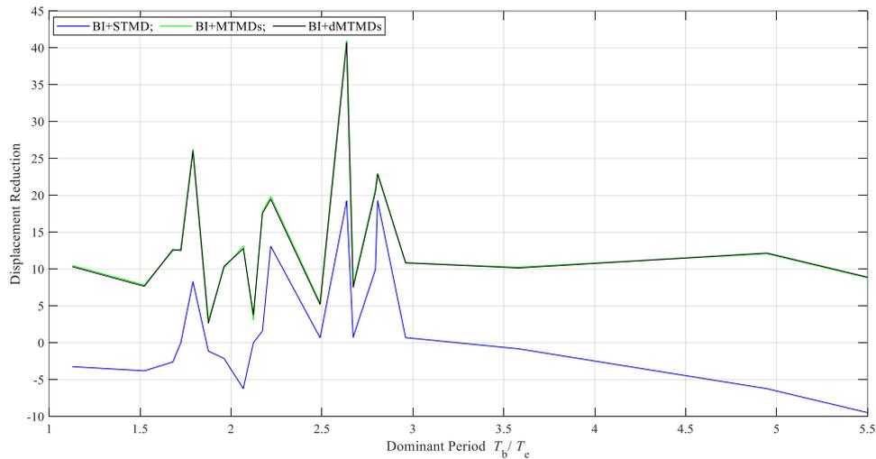
Fig. 5 – Variation of average reduction in bearing displacement for earthquakes with different dominant periods
