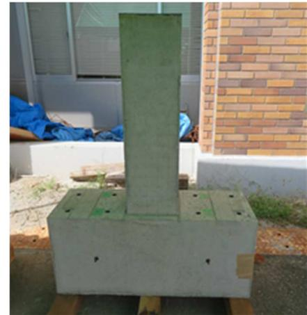
Fig. 3 – Configuration of the test specimen of RC column to set to the hydraulic actuator
