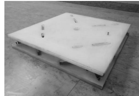
Seismic Isolator composed of linear rails TRC15
