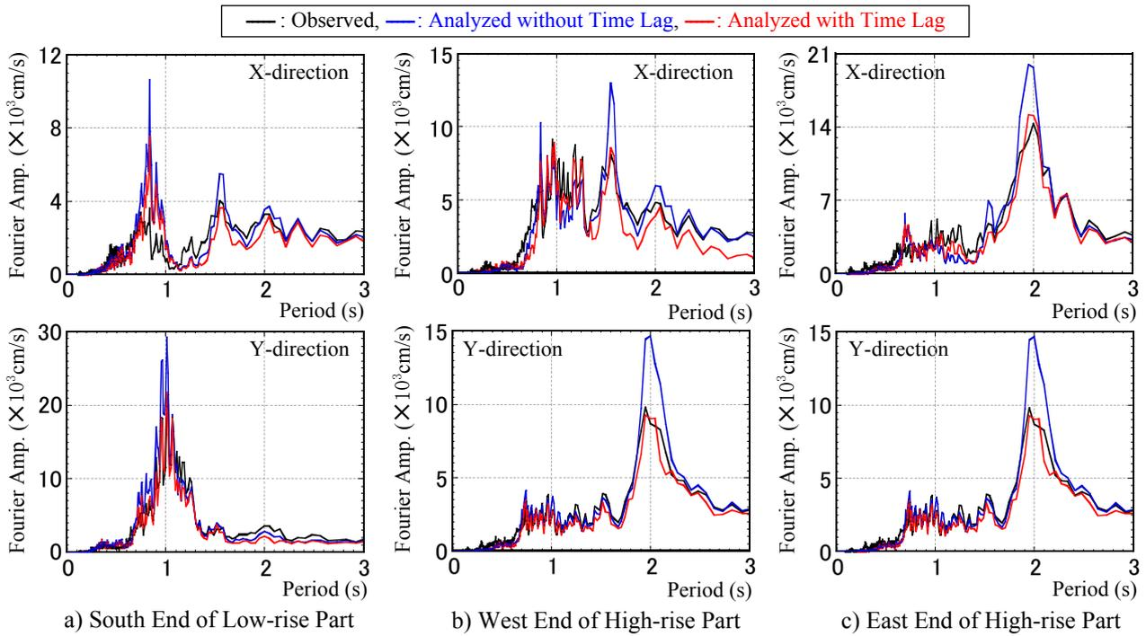
Fig.9 – Fourier Amplitude Spectra of Acceleration on Top Floor
