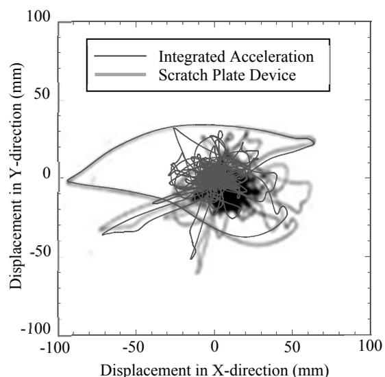
Fig.6 – Horizontal Orbit of Relative Displacement at Isolation Layer during "3.11 Earthquake"
