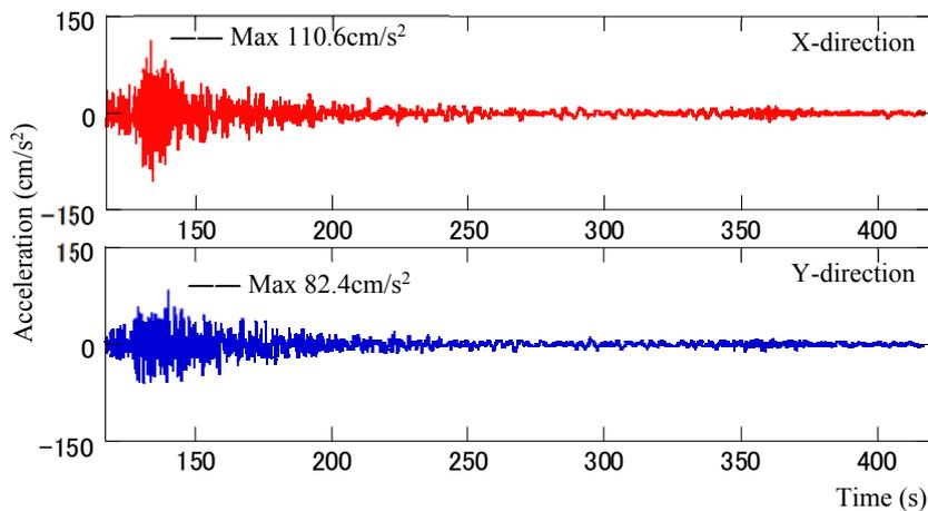
Fig.4 – Recorded Acceleration under Isolation Layer at West End of High-rise Part during "3.11 Earthquake" [No.004]
