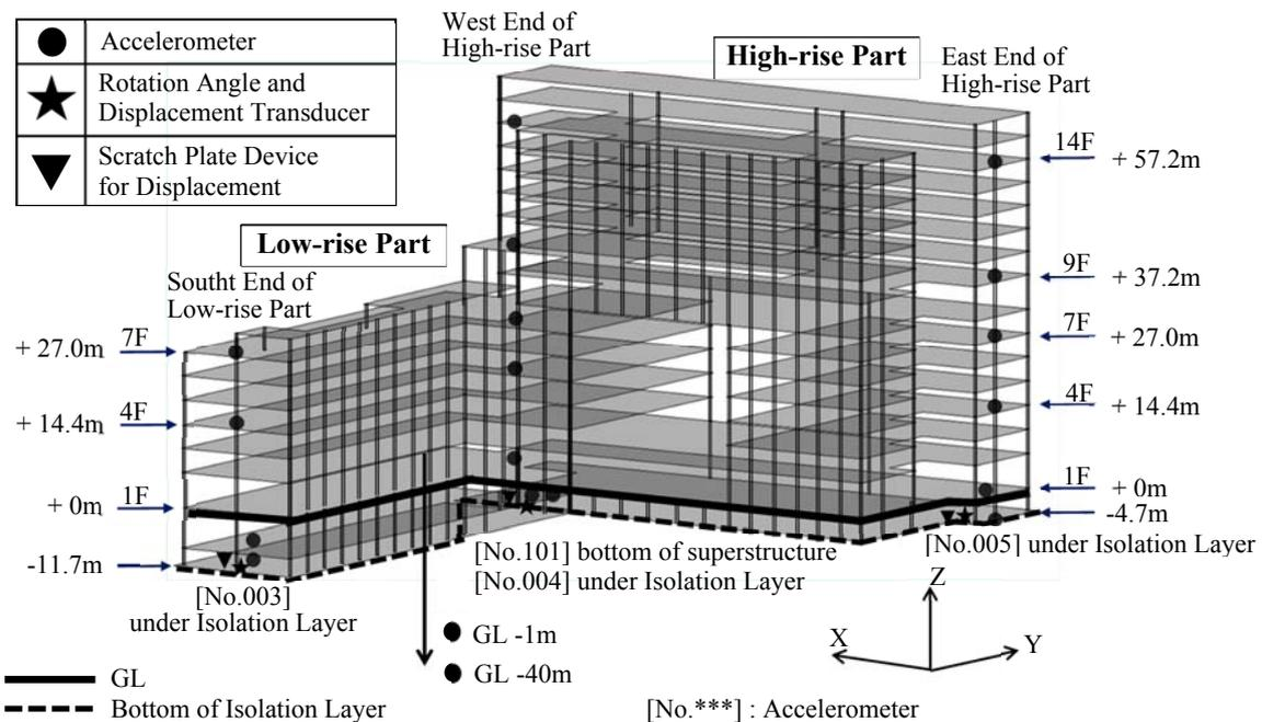
Fig. 2 – Layout of Sensors for Earthquake Response Observation
