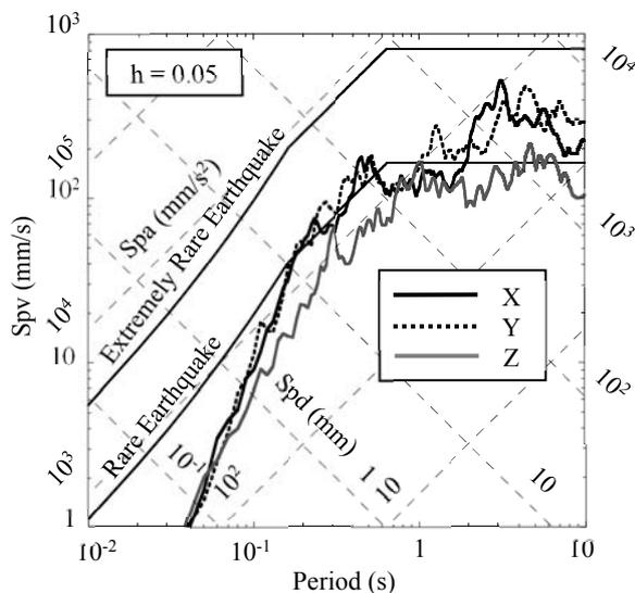
Fig.5 – Pseudo Response Spectra of "3.11 Earthquake" at GL-40m
