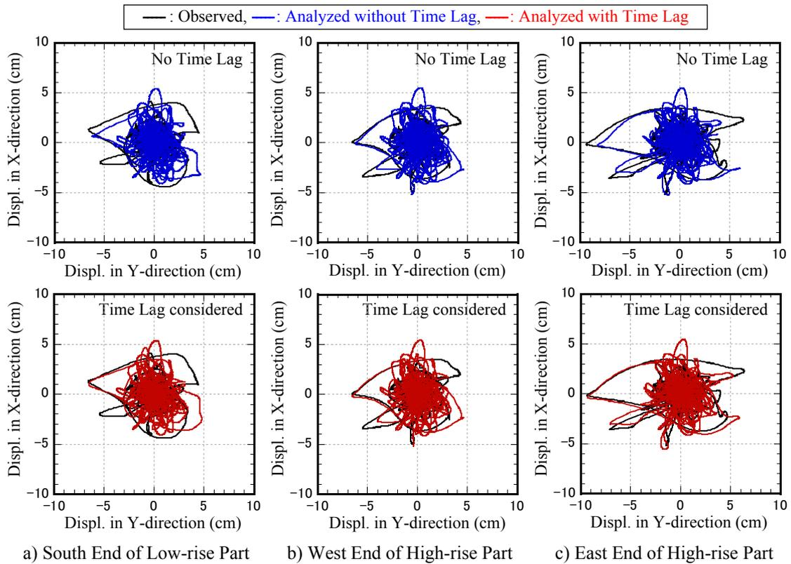
Fig.10 – Horizontal Orbits of Relative Displacement at Isolation Layer during "3.11 Earthquake"
