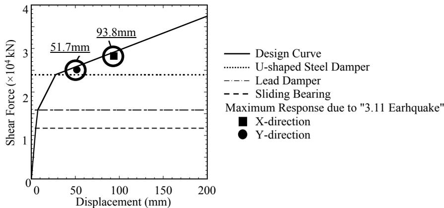
Fig.7 – Shear Force vs. Displacement at Isolation Layer
