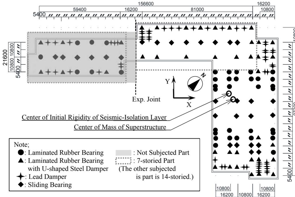
Fig. 1 – Location of Base Isolation Units
