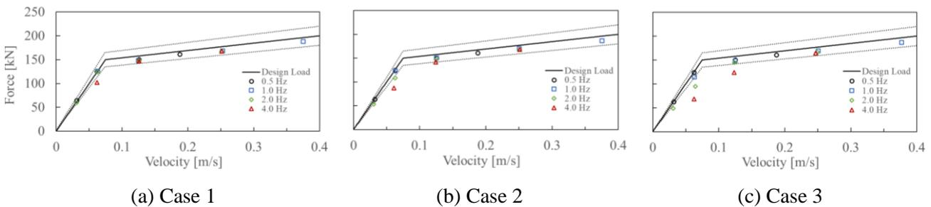
Fig. 5 - Damping force-velocity characteristics of damping device
