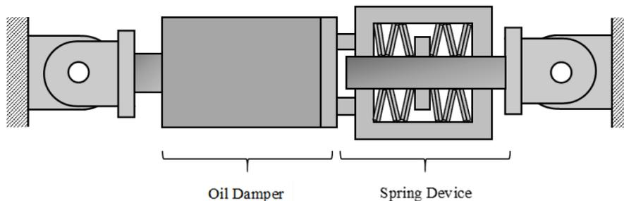
Fig. 1 - Conceptual diagram of damping device
