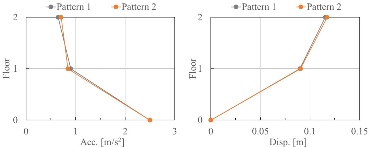
Fig. 11 - Maximum response in analyzed of seismic response
