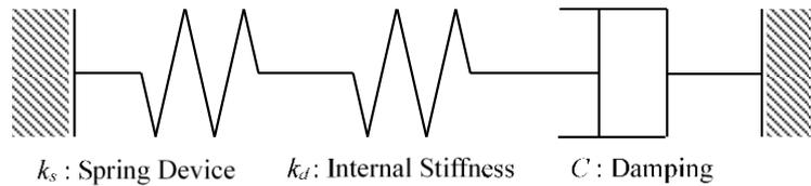
Fig. 7 - Equivalent stiffness of damping device
