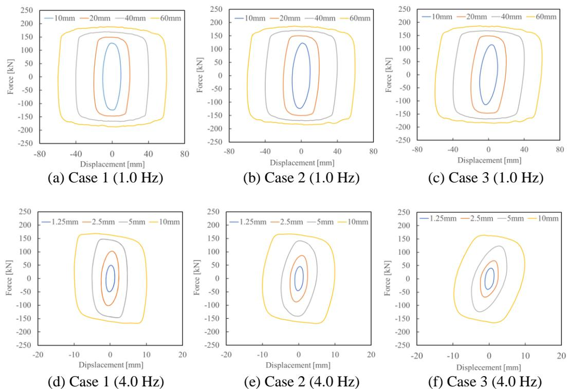
Fig. 4 - Load-displacement curve of damping device
