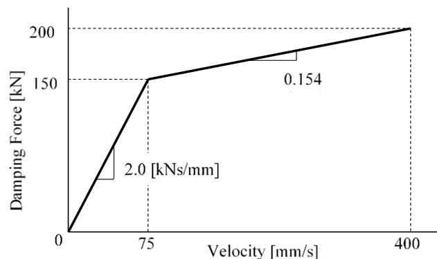
Fig. 3 - Relationship between force and velocity of oil damper
