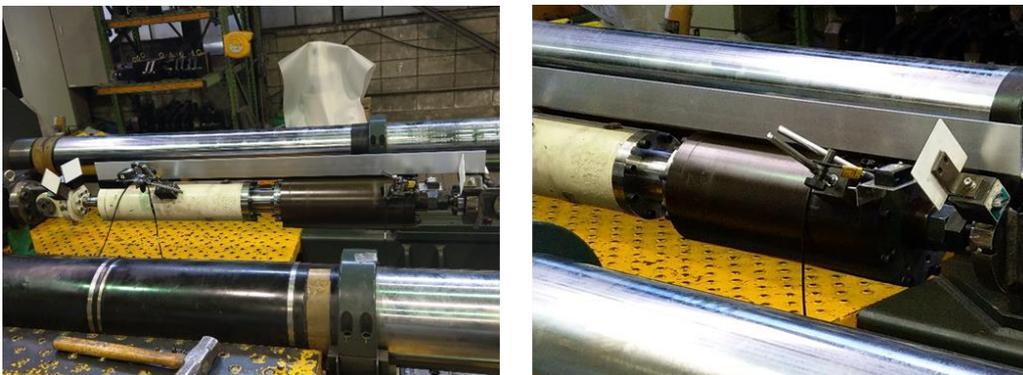
Fig. 2 - Damping device and spring device
