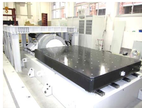
Fig. 3 – Actuator and shake table in Kobe University
