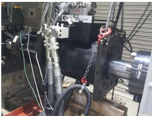
Fig. 3 – Actuator and shake table in Kobe University
