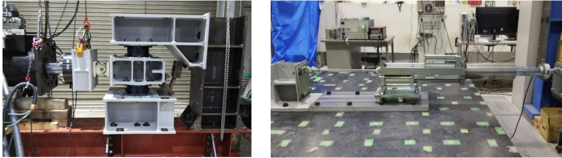
Fig. 4 – Isolated rubber bearings and MR damper used for DRTHS
