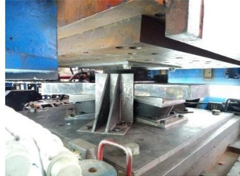
(a) Electro-hydraulic servo loading system
