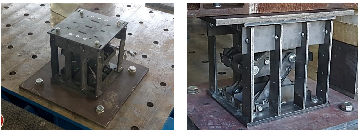
Fig. 2 – Kinematic Steel Joint (KSJ) isolator prototype.
