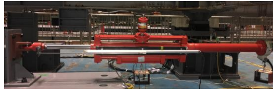
Photo 2 – MR damper installed in the base isolation layer
