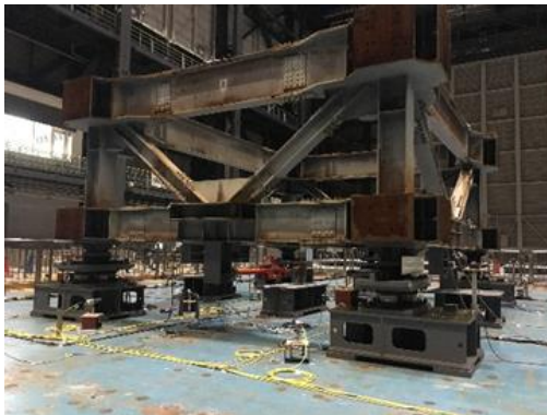
Photo 1 – Schematic view of E-Defense test
