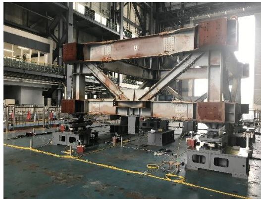
Fig. 5 – Overview of the base isolation specimen
