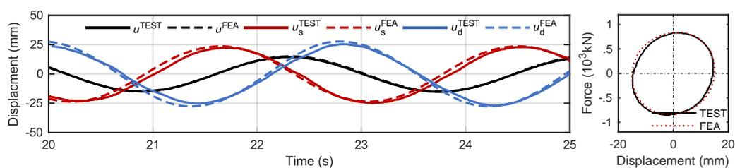
Fig. 8 – Comparison between test and FEA results
