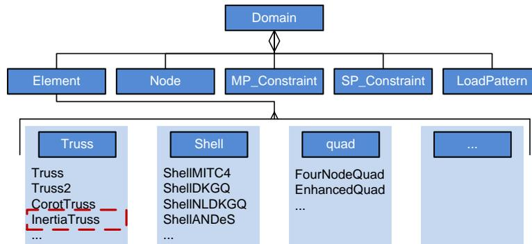
Fig. 6 – InertiaTruss class in OpenSees framework
