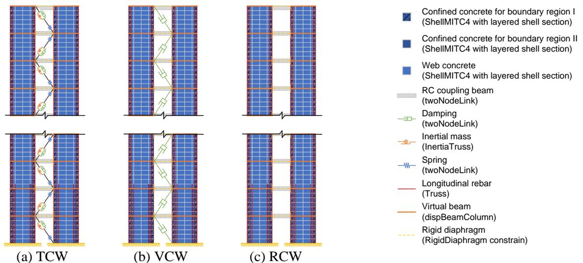
Fig. 9 – Schematic of models for nonlinear time history analysis
