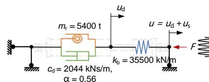
Fig. 7 – Schematic of the analytical model
