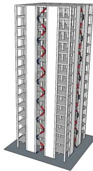
Fig. 1 – Schematic drawing of TVMD coupled wall system
