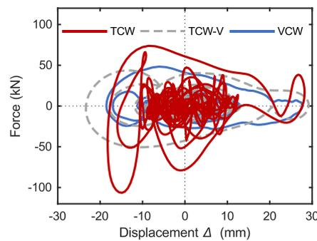
Fig. 15 – Hysteretic curves of the damper force (Victoria-Mexico earthquake @ DBE).
