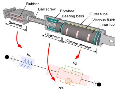
Fig. 5 – Finite element model of TVMD
