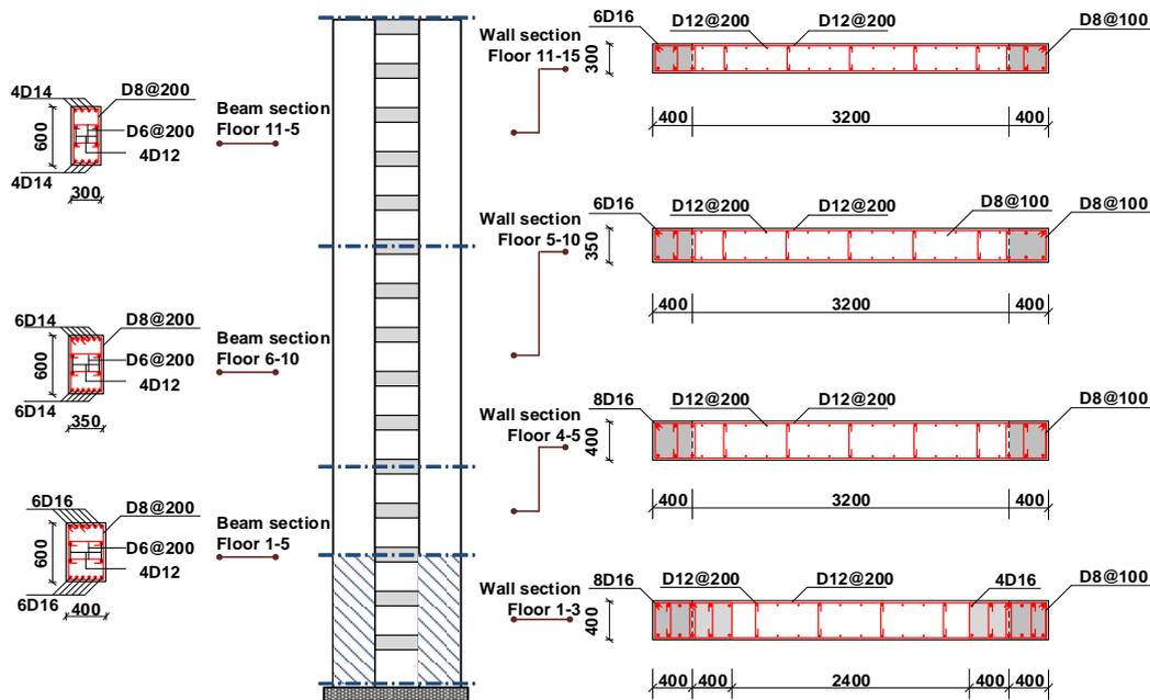
Fig. 4 – Wall dimensions and reinforcement details (unit: mm)
