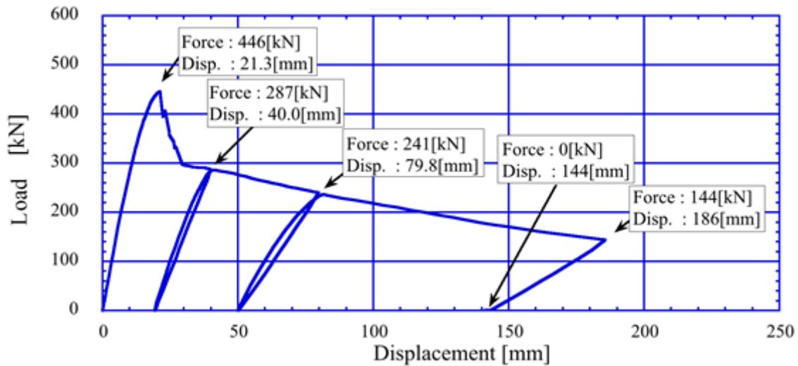
Fig. 5 – Reaction force of compression of experiment
