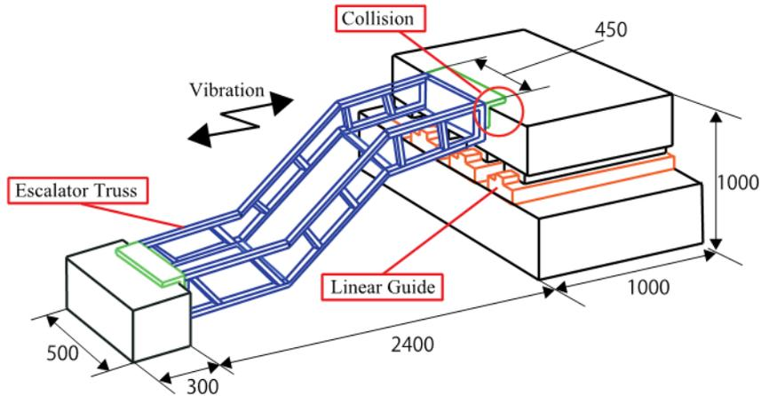
Fig.7 – Schematic of specimen
