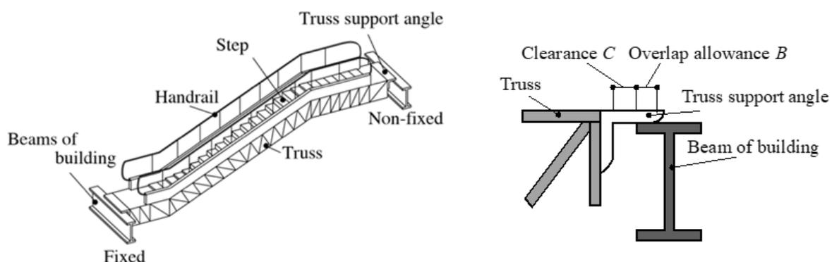
Fig. 1 – Escalator system and the non-fixed side of the escalator
