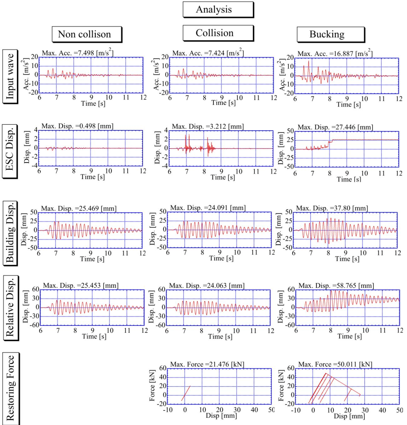
Fig. 11 – Seismic response analysis result
