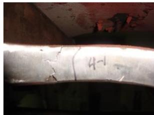
(a) Initial crack of inner ring (48mm)
