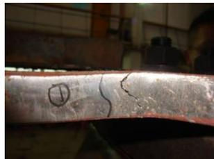
(a) Initial crack (180mm)
