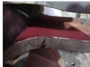
(b) Initial crack of outer ring (66mm)
