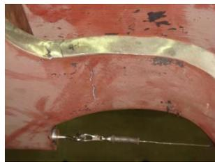
(c) Crack development of inner ring (84mm)
