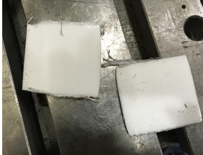
Fig. 7 – Delamination in PTFE specimens
