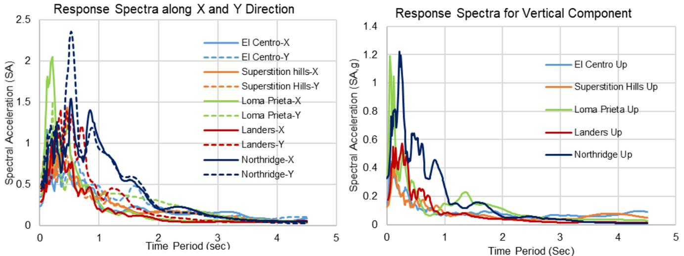
Fig. 5 – The response spectra (5% damped) of horizontal and vertical components of shallow crustal far field ground motions
