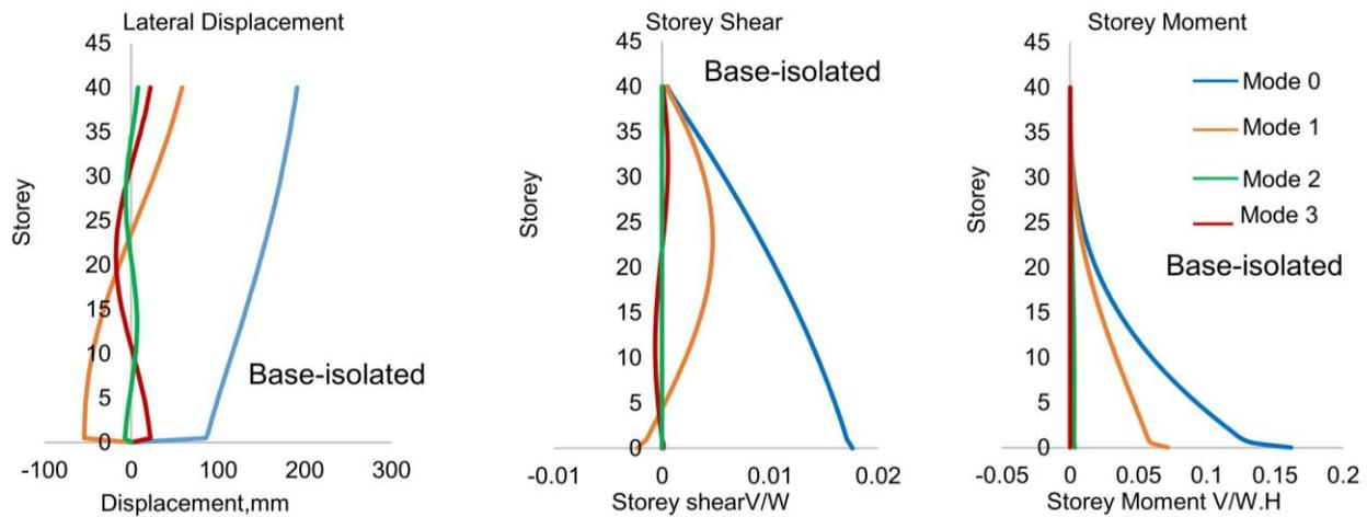
Fig. 7 – The comparison of modal demands for fixed-base and base-isolated systems
