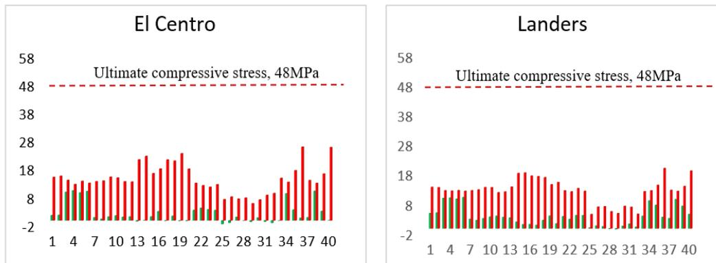
Fig. 10(c) – The axial compressive stress in bearings after applying the mitigation technique
