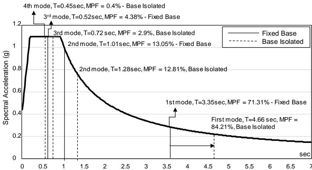
Fig. 6 – The natural time periods of fixed-base structure and base-isolated structure
