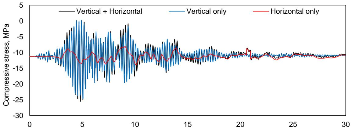
Fig. 9 – The axial stress in Beaming #12 under different cases of ground motion components
