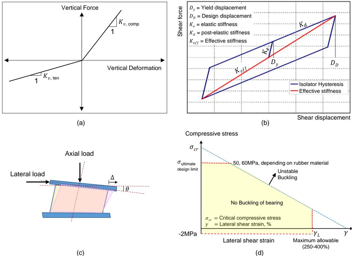
Fig. 2 – (a) The vertical properties, and (b) horizontal properties of the lead core rubber bearings. (c) the induced shear deformation due to rotation, (d) the ultimate property diagram for lead core rubber bearings
