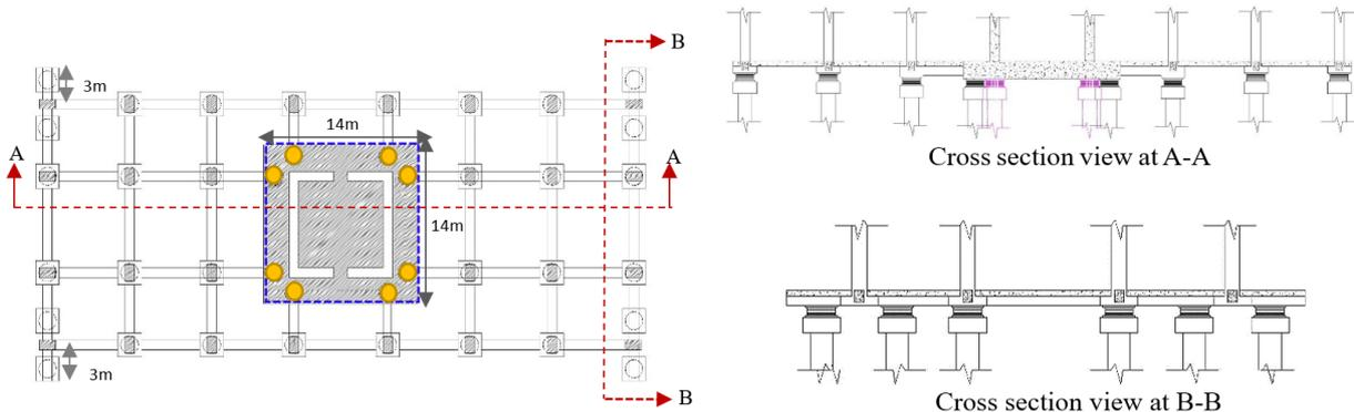
Fig. 10(b) – The plan layout and cross-section view at isolation level
