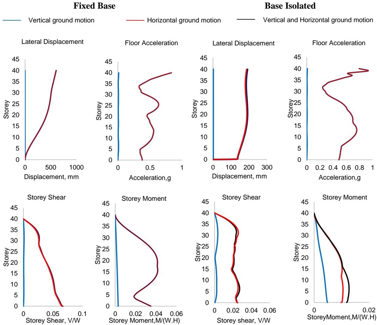
Fig. 8 – The comparison of lateral displacement, floor acceleration, storey shear and storey moment for fixed base and base isolated cases for effect of vertical and horizontal components of ground motions
