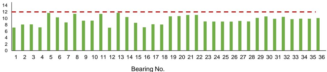
Fig. 4 – The pre-compressive load in bearings under the service load condition
