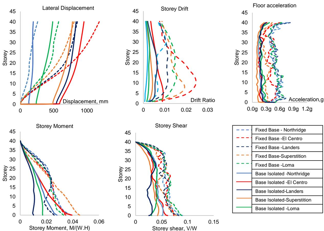
Fig. 11 – The comparison of total inelastic seismic demands of fixed-based (broken line) and base-isolated (solid line) buildings subjected to 5 input ground motions
