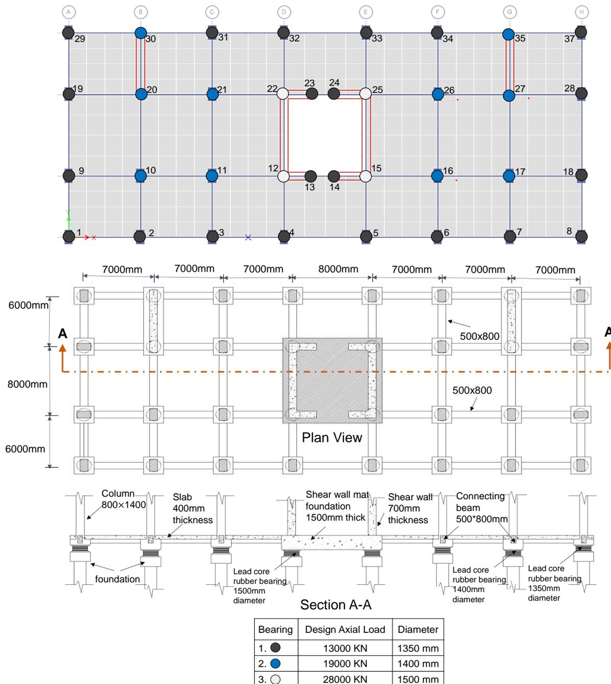
Fig. 3 – The layout of bearings with numbers in structural plan view and the section view at isolation level
