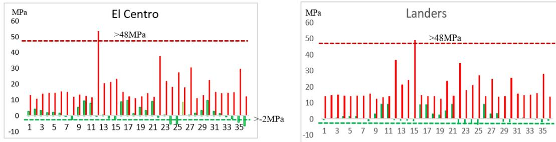
Fig. 10(a) – Axial reaction in bearings (bearing numbers are shown in Fig. 3)
