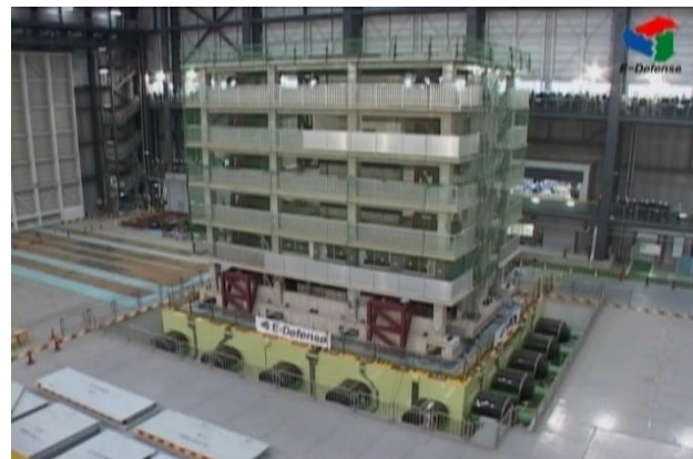
(b) Six-story reinforced concrete building excitation test
