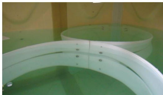
Photo 3 Installation situation of 8-shaped floating damping device
