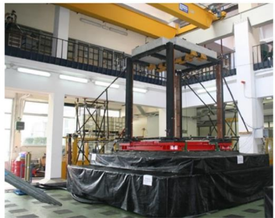
Fig. 7 – (a) Cabinet projection of the prototype building and the instrumentation set-up; (b) view of the test frame of the shaking table at the DiST laboratory University of Naples Federico II [16]
