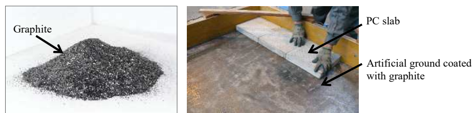
Photo 1 – Friction material (graphite) and sliding faces
