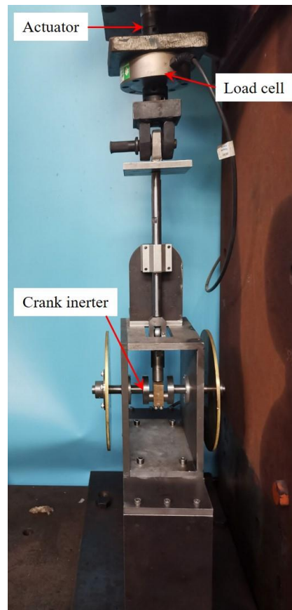
Fig. 3 Photograph of experimental setup for crank inerter test
