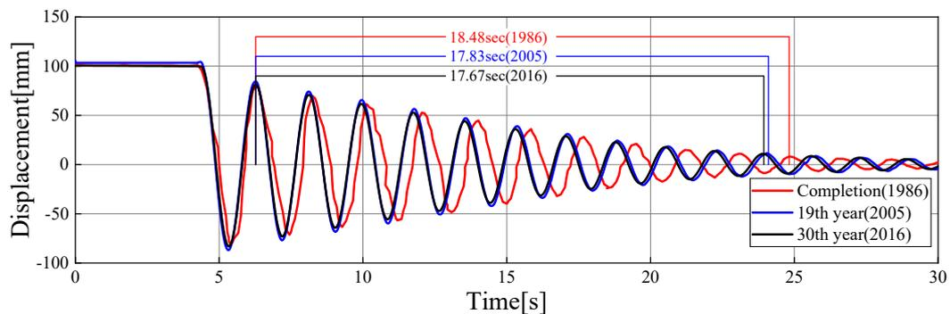
Fig. 7 – Time history waveforms of displacement (Free vibration test)
