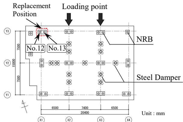
Fig. 1 – Plane of seismic isolation devices
