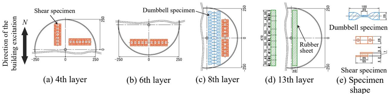
Fig. 16 – Position of rubber specimen cut from the removed bearing
