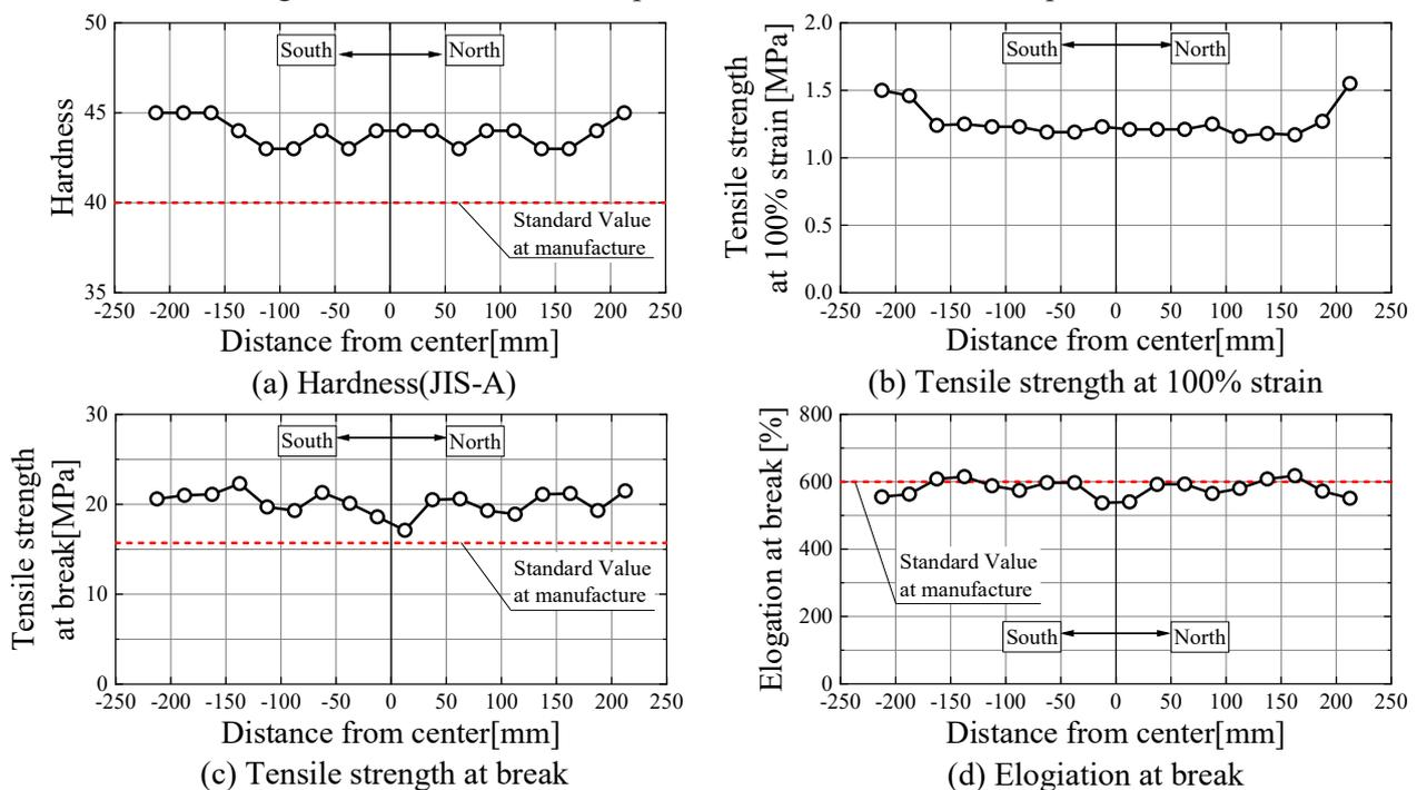
Fig. 18 – Results of dumbbell specimen(8th layer in the removed bearing)
