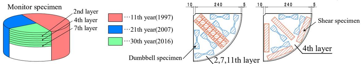
Fig. 17 – Position of rubber specimen cut from the monitor specimen
