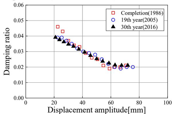
Fig. 9 – Comparison of damping ratio
