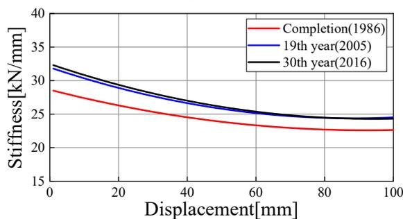
Fig. 5 – Stiffness of the laminated rubber bearings at each displacement
