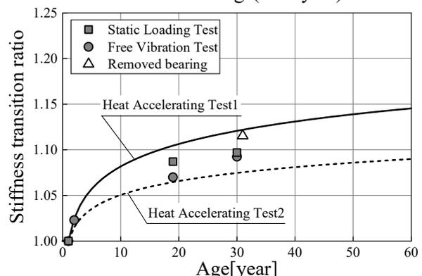
Fig. 12 – Stiffness transition ratio of age deterioration
