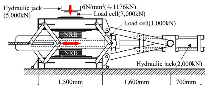
Fig.3 – Loading system of bearing element
