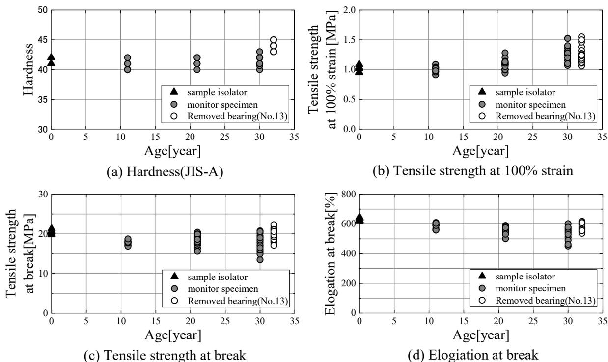
Fig. 21 – Comparison of dumbbell test results
