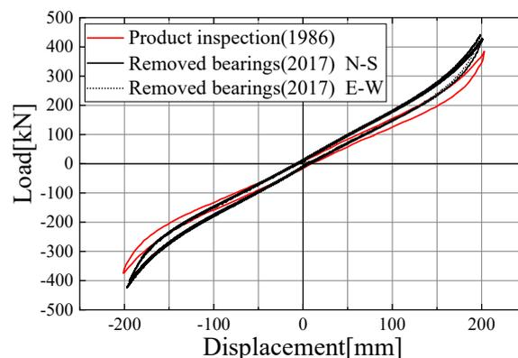
Fig. 10 – Relation between load and displacement of removed bearings(3rd cycle)
