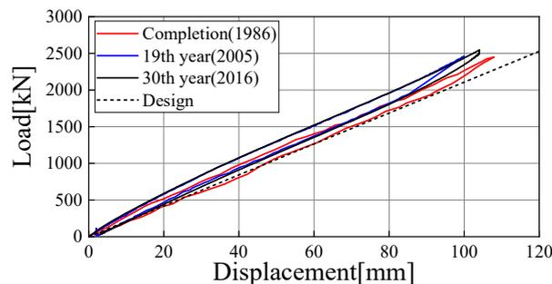
Fig.4 – Relation between load and displacement by static test
