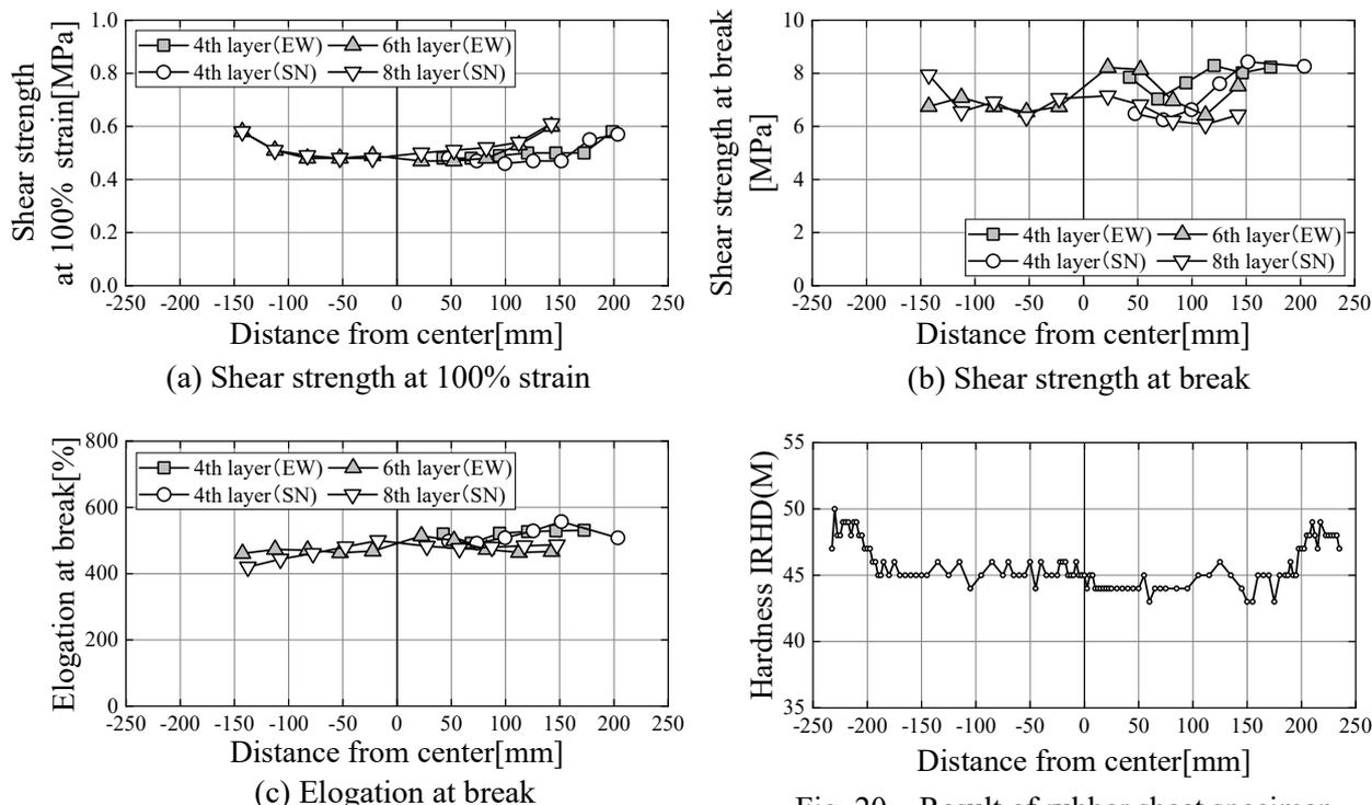
Fig. 19 – Result of shear test specimen
