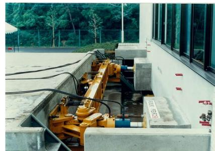
Photo 2 – Loading device installation
