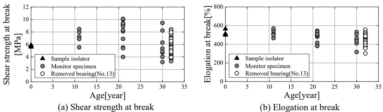
Fig. 22 – Comparison of shear test results
