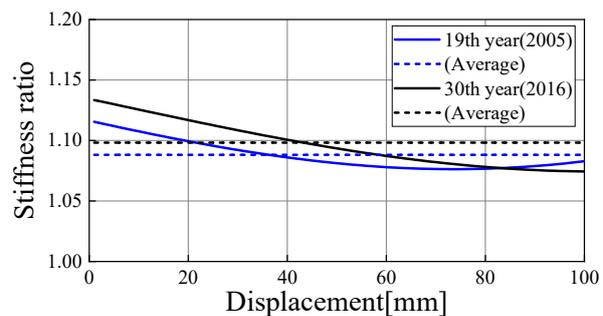
Fig. 6 – Stiffness ratio of the time of construction to aging
