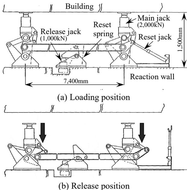
Fig.2 – Loading device of the building
