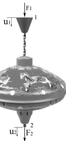
Fig. 1 – A physical realization of the inertor in which the force output is proportional only to the relative acceleration of nodes 1 and 2 and is the mechanical analogue of the capacitor in a force current/velocity-voltage analogy
