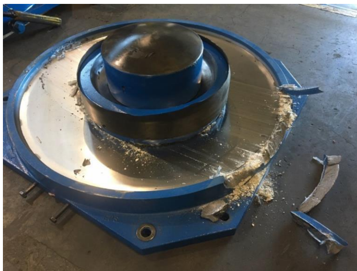
Fig. 6 – Full scale TFP isolator after ultimate capacity test
