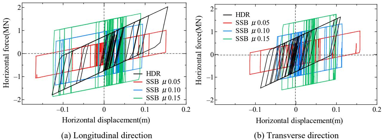
Fig. 4 – Horizontal force-displacement hysteresis loops of bearing on P1
