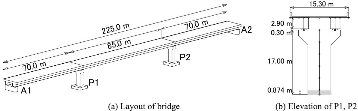
Fig. 1 – Schematic diagram of bridge
