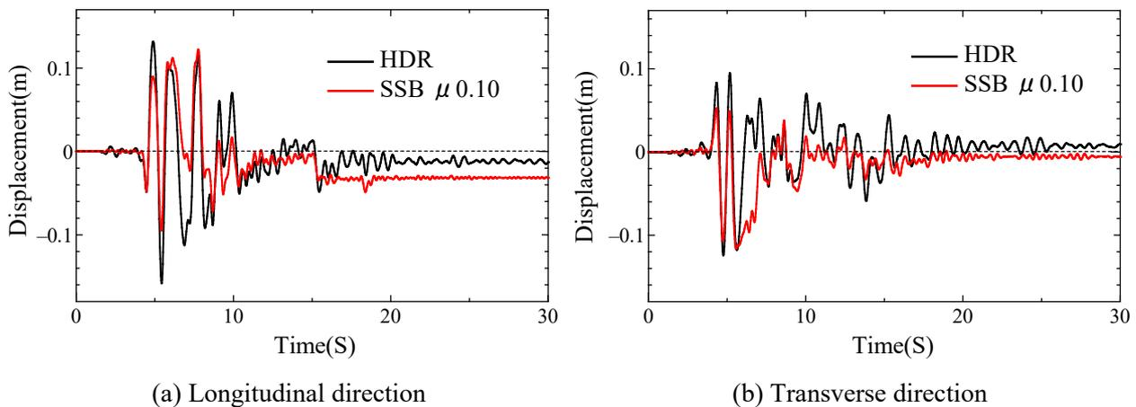
Fig. 5 – The time history displacement response of superstructure on P1
