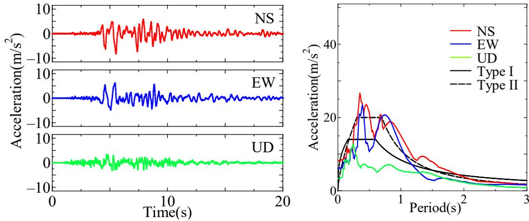
(a) Recorded ground motions of JMA Kobe (b) Acceleration response spectra (for 5% damping)
