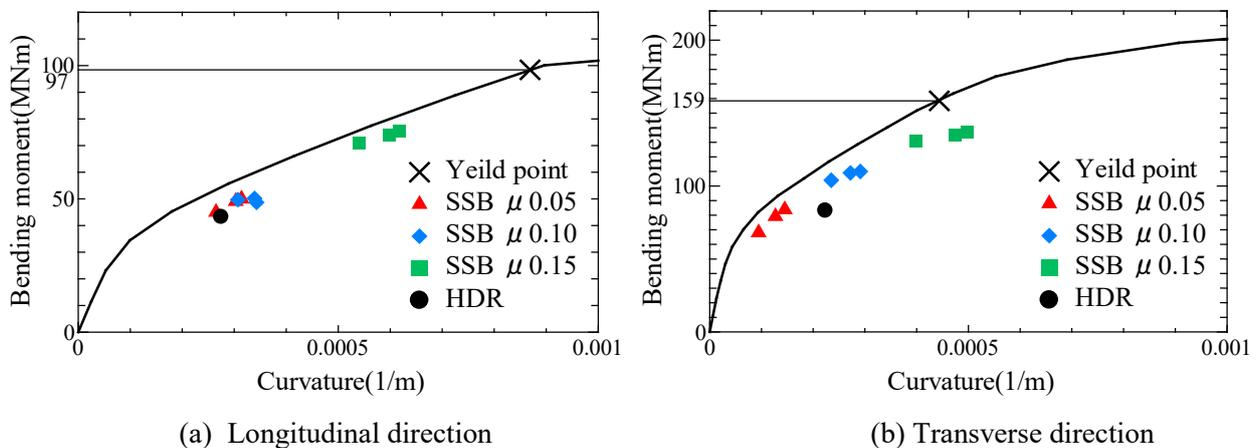
Fig. 6 – Maximum bending moment-curvature relationship of plastic hinge of P1
