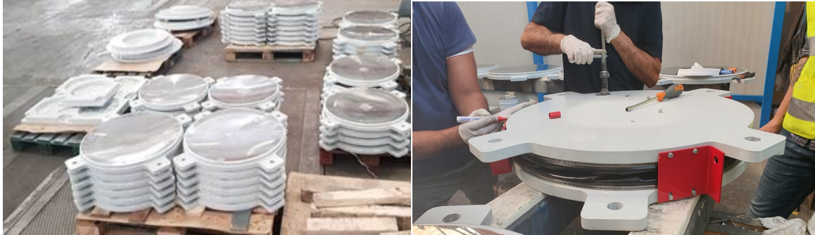
Fig. 15 – Sliding plates (top) and final quality control checks of the assembled device (down)
