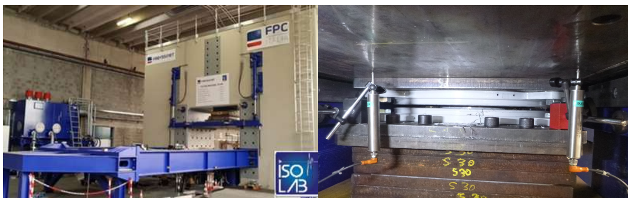
Fig. 10 – 70 MN ISOLAB Testing Machine (left) and ISOSISM ® PS 3300/700 under the press (right)
