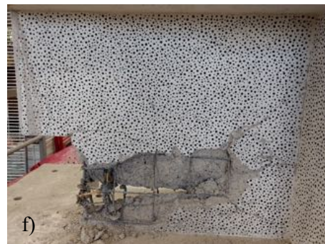
Figure 8. a) Load-displacement curve for ET1. b) Buckling of unrestrained reinforcement (end of test), c) Load-displacement curve for ET2. d) Spalling of concrete cover at 1.6 %. e) Load-displacement curve for ET3. f) Damage in the whole web.
